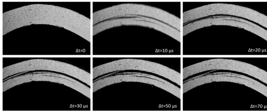
Figure 9: High speed photos of TPNCF2 specimen 2nd test (2nd batch), taken at 100,000 fps showing the failure sequence.
