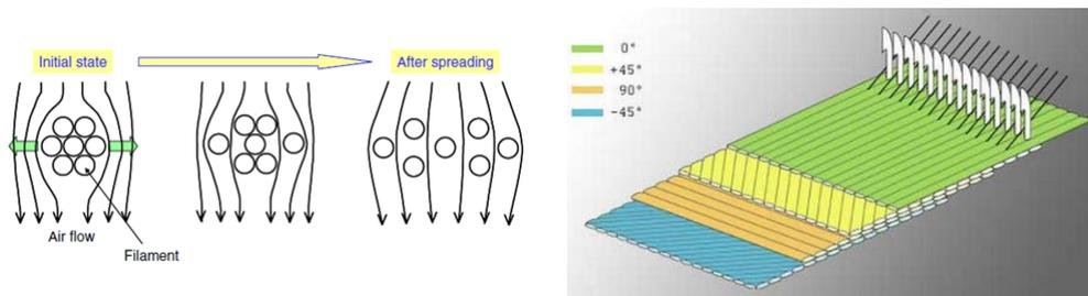
Figure 1: *schematic of (a) tow-spreading process (b) ENF test, (c) Ply combining process during manufacturing*
