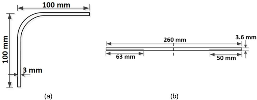
Figure 2: Specimen geometry of thin fiber NCF used for (a) 4-point bending tests and (b) fracture toughness tests.
