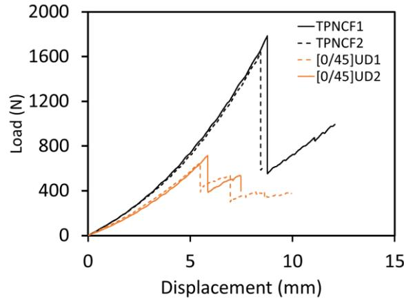
Figure 7: Four point bending load displacement curves of [0] UD, [0/45] UD and [0/45] thin fiber NCF laminates all together.
