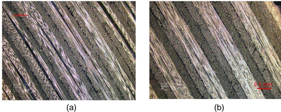
Figure 3: Microscopic side view  $[0/45/-45/0]$  (a) thin ply NCF laminate, (b) conventional thicker ply laminate.
