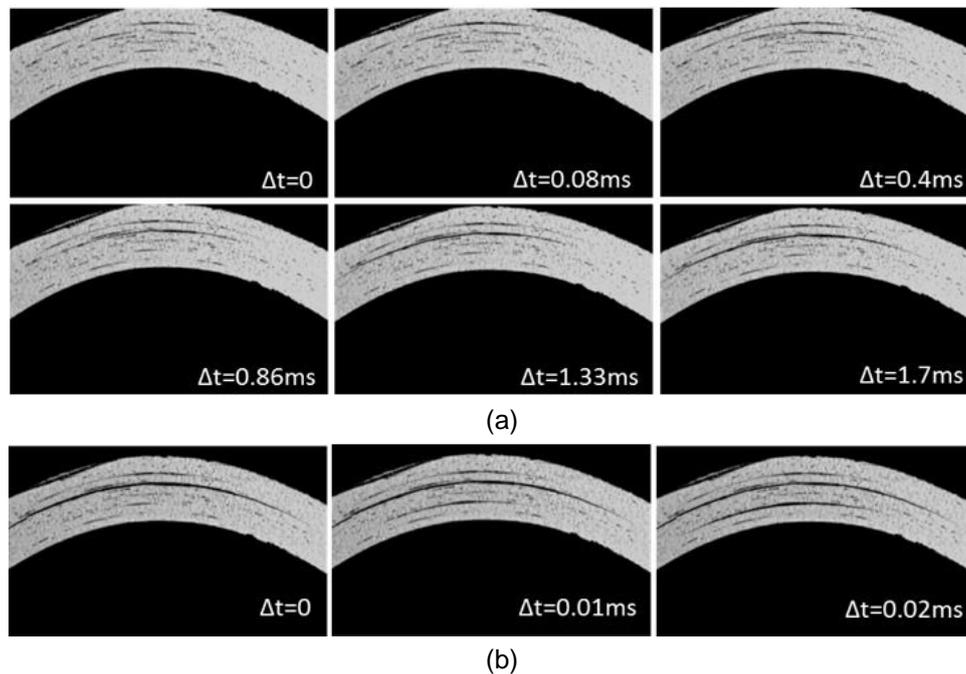
Figure 8: HSC photos taken at 100,000 fps for UD2 laminate corresponding at (a) first and (b) second load drop, respectively.
