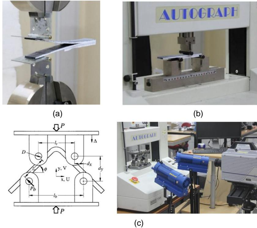
Figure 4: *Experimental Setup for (a) double cantilever beam test (b) ENF test, (c) curved beam strength test of L-shaped laminate*
