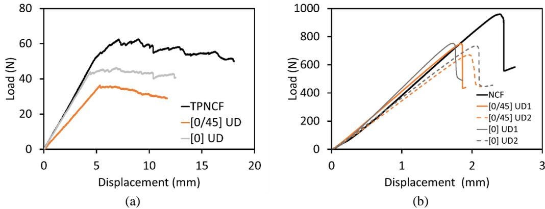
Figure 5: Load displacement curves of NCF, [0/45] UD and [0] UD laminates obtained (a) DCB tests and (b) ENF tests.
