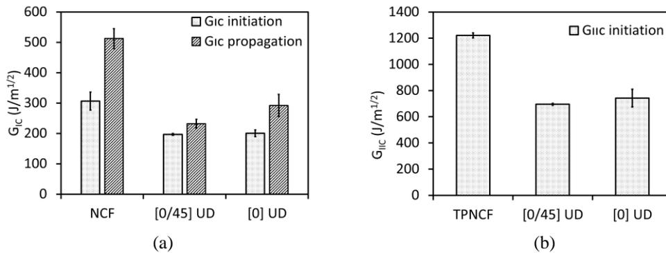
Figure 6: (a) Bar graph of Mode-I fracture toughness ( $G_{IC}$ ) initiation and propagation values obtained by MBT and (b) bar graph of Mode-II fracture toughness values calculated by direct beam theory for TPNCF, [0] UD and [0/45] UD laminates.
