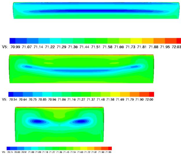
Figure 9: Surface pressure contours on the lower surface of three wings with aspect ratios of 10, 5 and 2.5 (Case 2 of Table 1)
