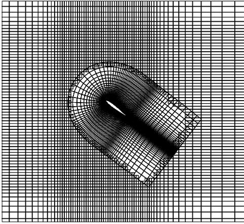
Figure 2: Grid system used in 2-D flow computation
