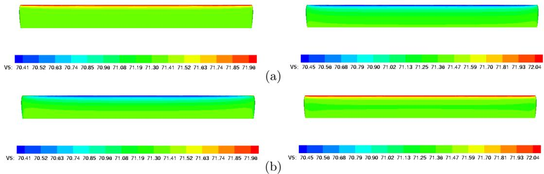
Figure 6: Surface pressure contours on the lower (a) and upper (b) surfaces at two instances during the cycle. The formation of a vortical structure on the surface is evident (Case 3 of Table 1)
