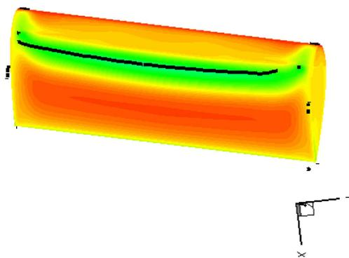
Figure 7: Vortex core extracted from the CFD solution for Case 1 of Table 1
