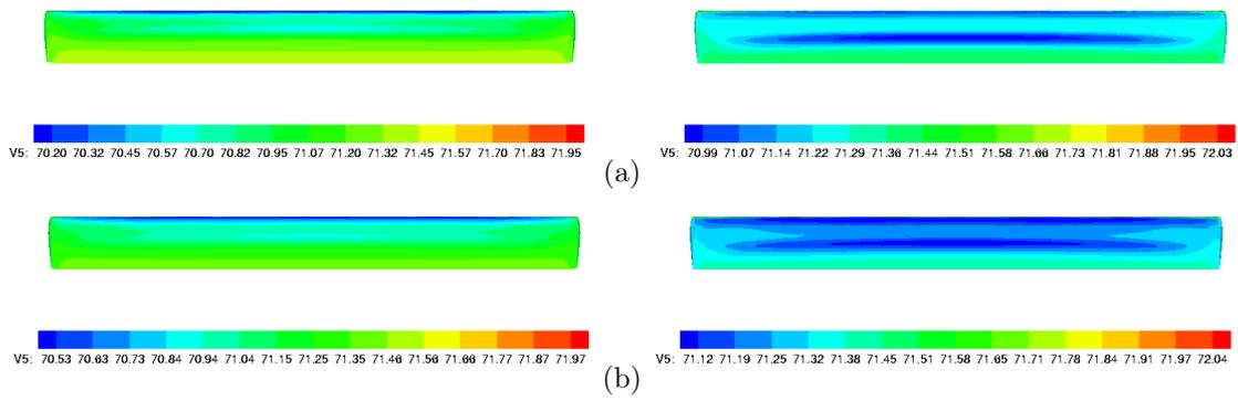
Figure 4: Surface pressure contours on the lower (a) and upper (b) surfaces at two instances during the cycle. The formation of a vortical structure on the surface is evident (Case 1 of Table 1)
