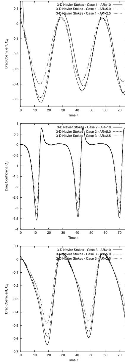
Figure 3: Effect of aspect ratio on thrust for the datum, thrust and efficiency cases of Table 2.
