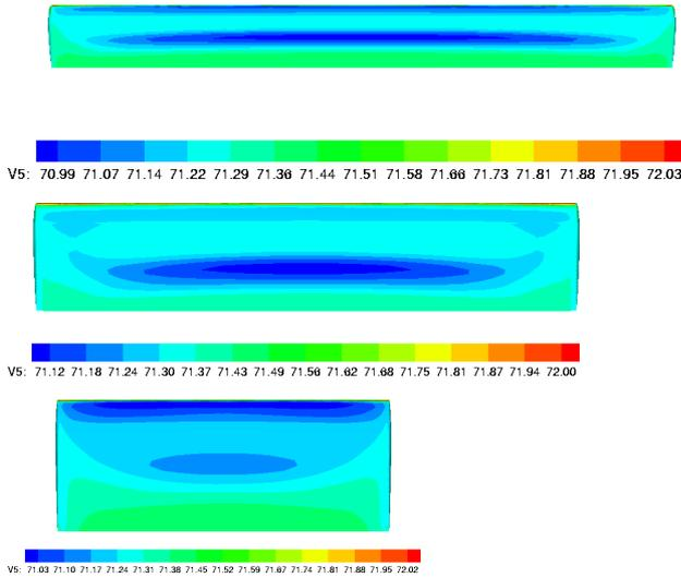
Figure 8: Surface pressure contours on the lower surface of three wings with aspect ratios of 10, 5 and 2.5 (Case 1 of Table 1)
