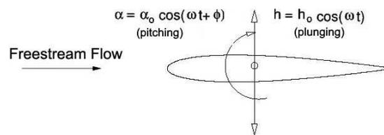
Figure 1: Flapping motion of an airfoil
