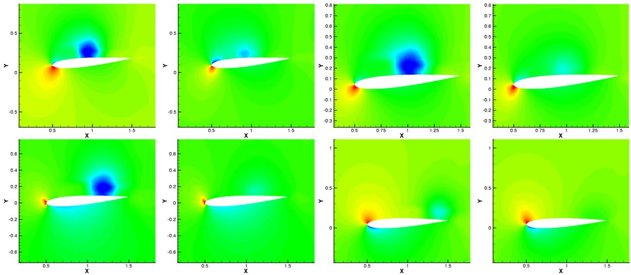
Figure 12: Pressure contours for case 1 of Table 2, showing the evolution of the vortex during the upstroke cycle. Two slices are shown corresponding to (a) the mid-span of the wing and (b) the near-tip region.
