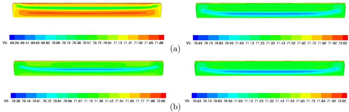
Figure 5: Surface pressure contours on the lower (a) and upper (b) surfaces at two instances during the cycle. The formation of a vortical structure on the surface is evident (Case 2 of Table 1)
