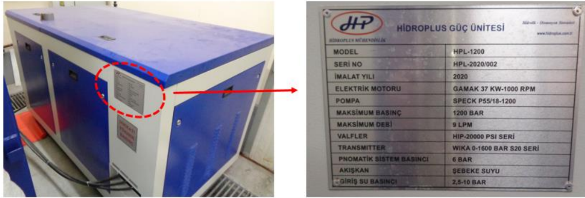
Figure 19. Pressure Test Unit
