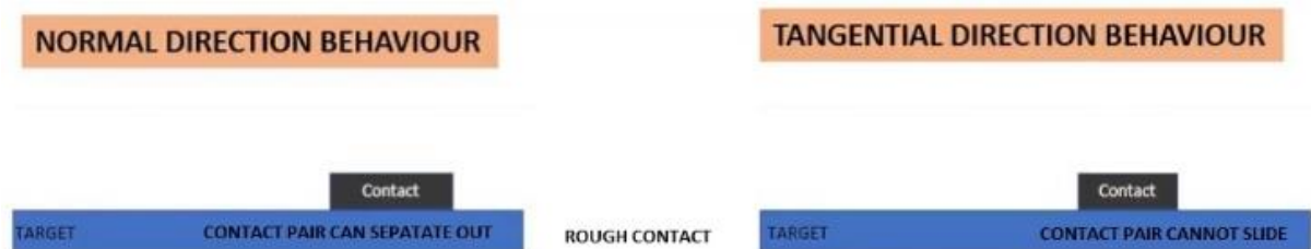
Figure 10. Rough connection type
