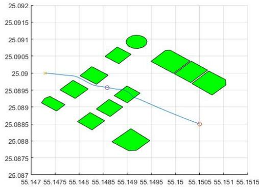
(a) Trajectory in 2-D with Static Obstacle.
