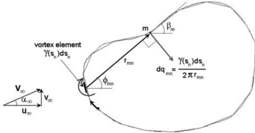
Figure 2: Surface representation of an arbitrary geometry in a panel method using straight line segments and the velocity induced at m by a surface vortex element at n. [Uzol et al. [2010]]
