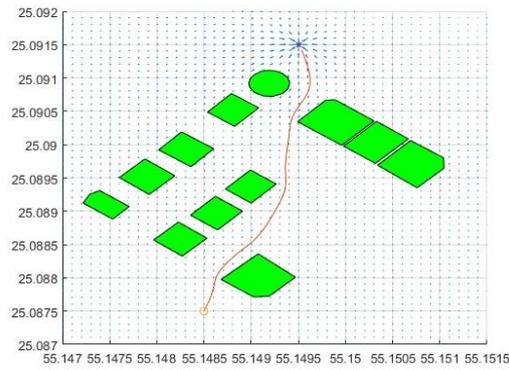
(c) Streamlines and Trajectory of Vehicle 3.
