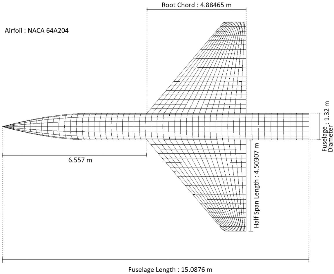
Figure 3: General geometric properties of F-16 aircraft
