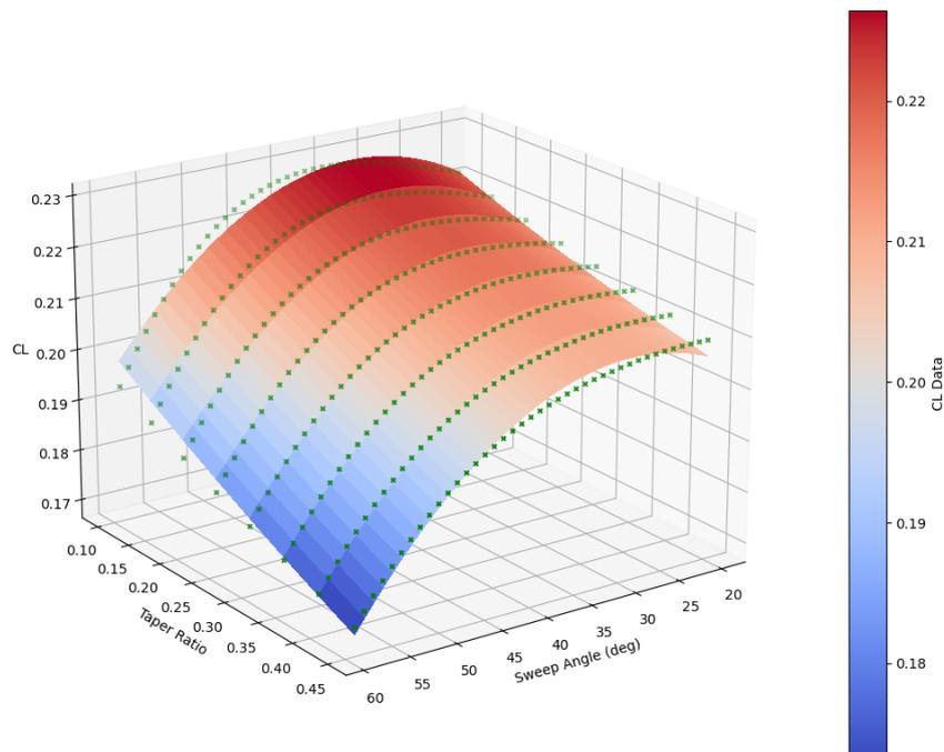
Figure 8: The effect of the taper ratio and sweep angle on lift coefficient
