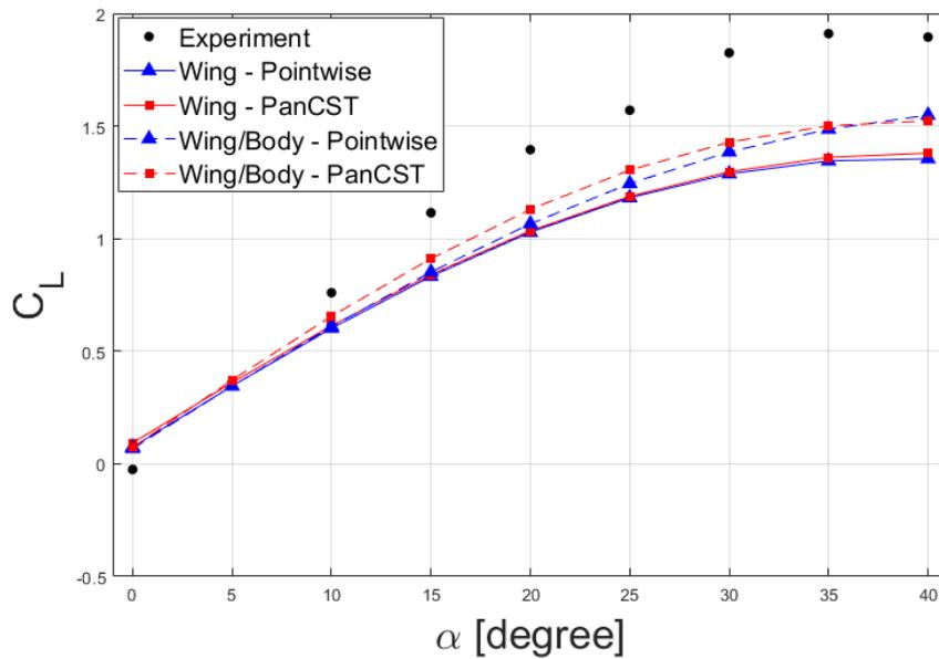
Figure 6: Comparison of lift coefficient between experiment data and Pointwise & panCST results
