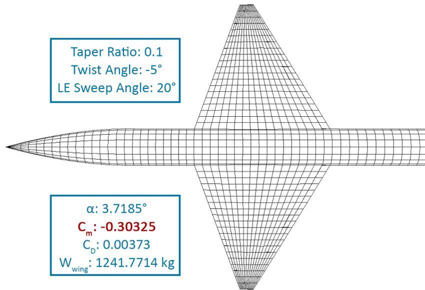
Figure 15: The aircraft geometry where the moment coefficient is minimum
