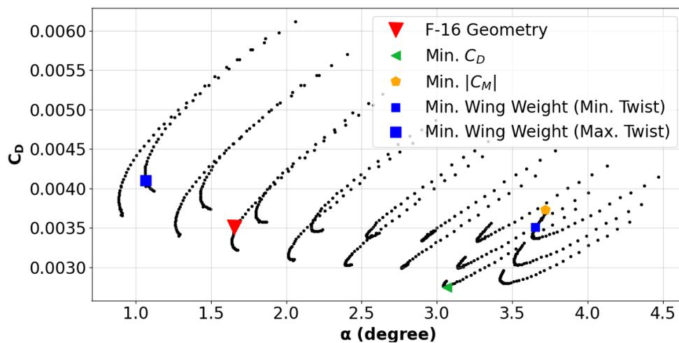
Figure 11: Drag coefficients and corresponding angles of attack for geometries
