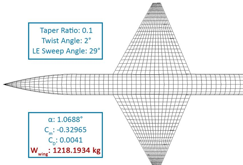
Figure 16: The aircraft geometry where the wing weight is minimum
