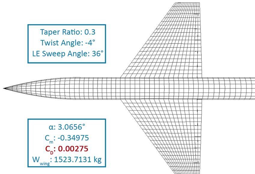
Figure 14: The aircraft geometry where the induced drag coefficient is minimum
