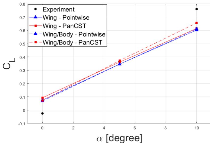
Figure 7: Comparison of lift coefficient between experiment data and Pointwise & panCST results for lower angles
