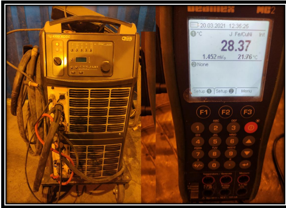
Figure 3: Welding machine and temperature calibrator
