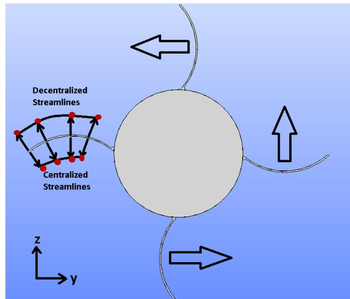
Figure 1. Wrap-around Tail Fin Roll Induction Mechanism
