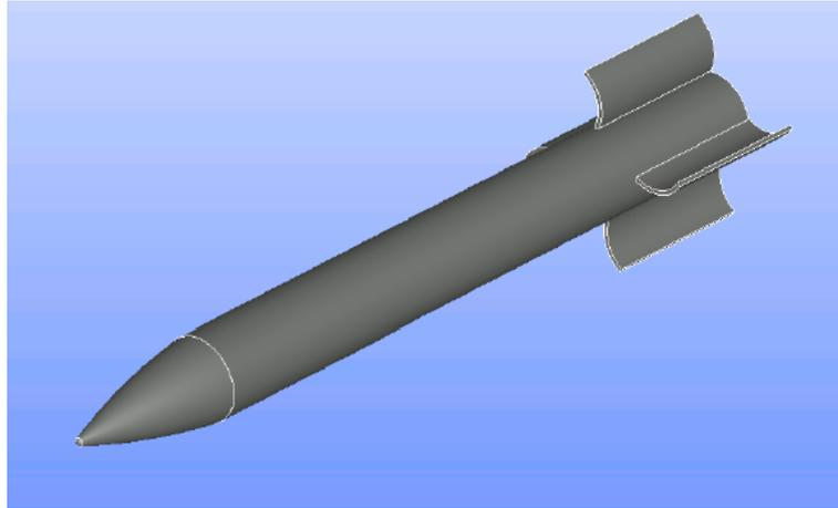
Figure 2. The Dahlke's wrap-around tail finned missile [Dahlke 1976]
