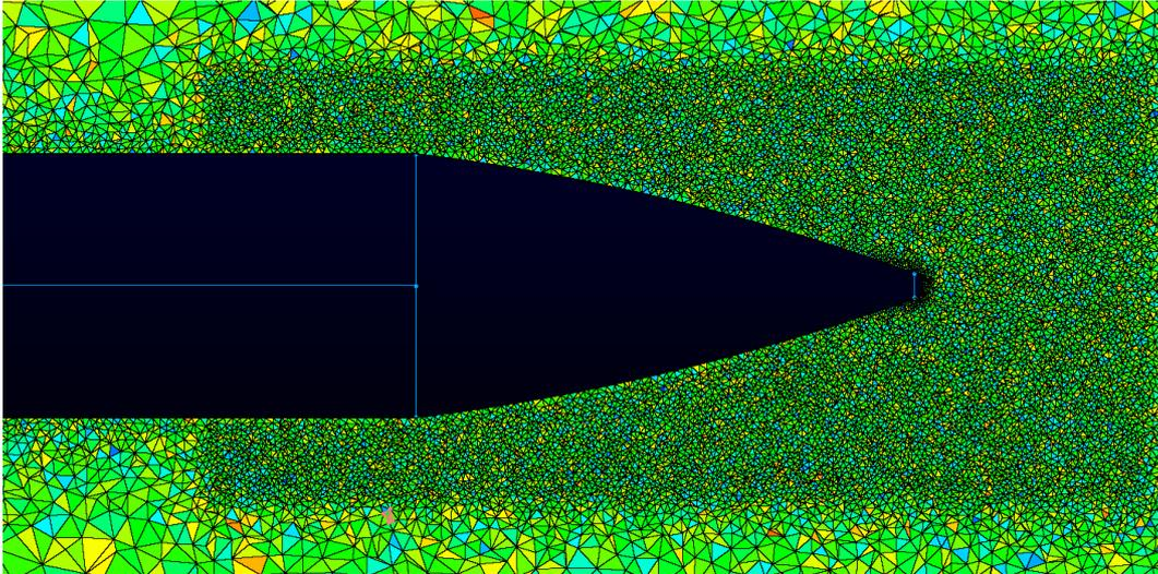
Figure 7: Locally refined regions around the missile head
