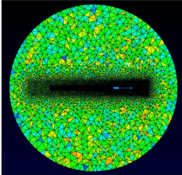
Figure 4: Spherical Computational Domain and Unstructured Grid
