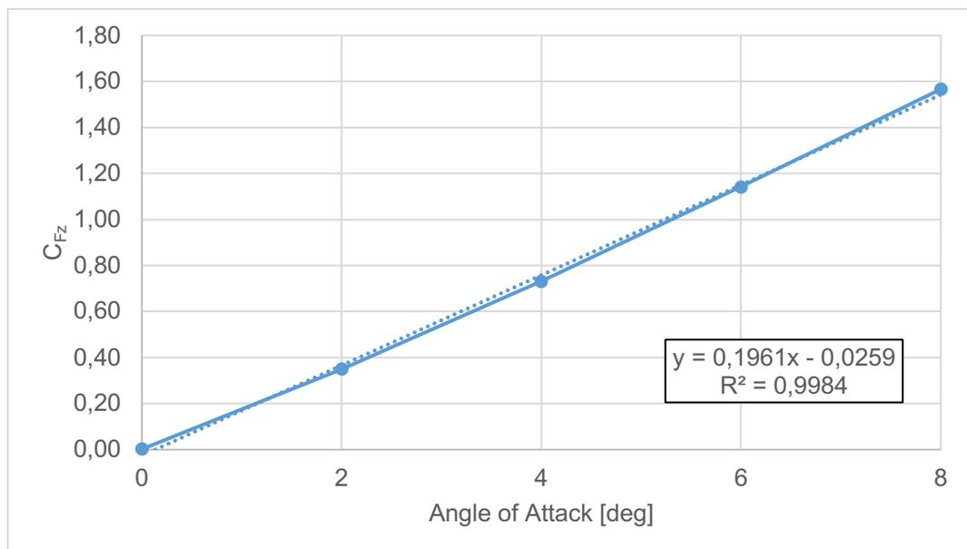
Figure 13. Normal Force Coefficient versus Angle of Attack
