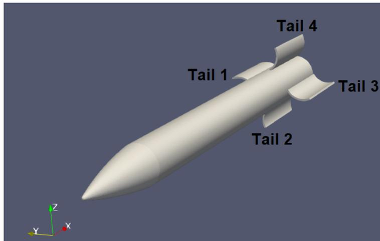
Figure 12: The numbering and names of wrap-around tail fins
