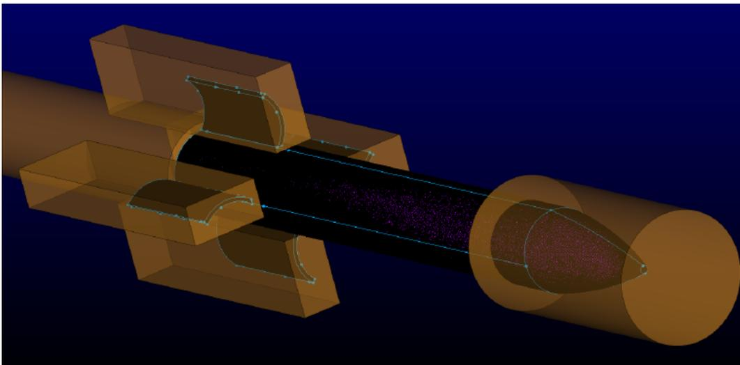
Figure 5: Grid refinement regions around the missile
