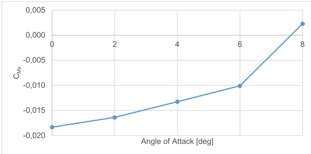
Figure 14. Roll Moment Coefficient versus Angle of attack
