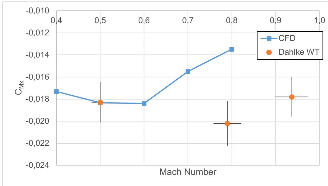
Figure 9. Comparison of Computational Results with Wind Tunnel Data: Roll Moment Coefficient versus Mach Number
