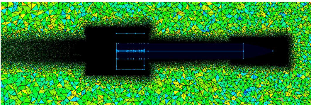
Figure 6: Unstructured grid around the missile with grid refinement regions
