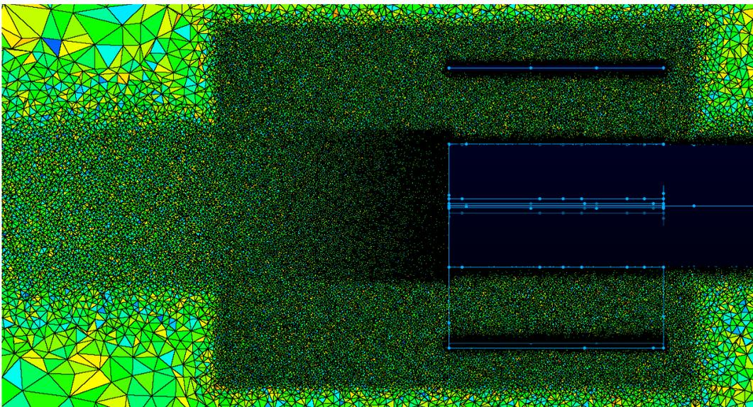
Figure 8: Locally refined regions around the tail fins and in the missile wake region
