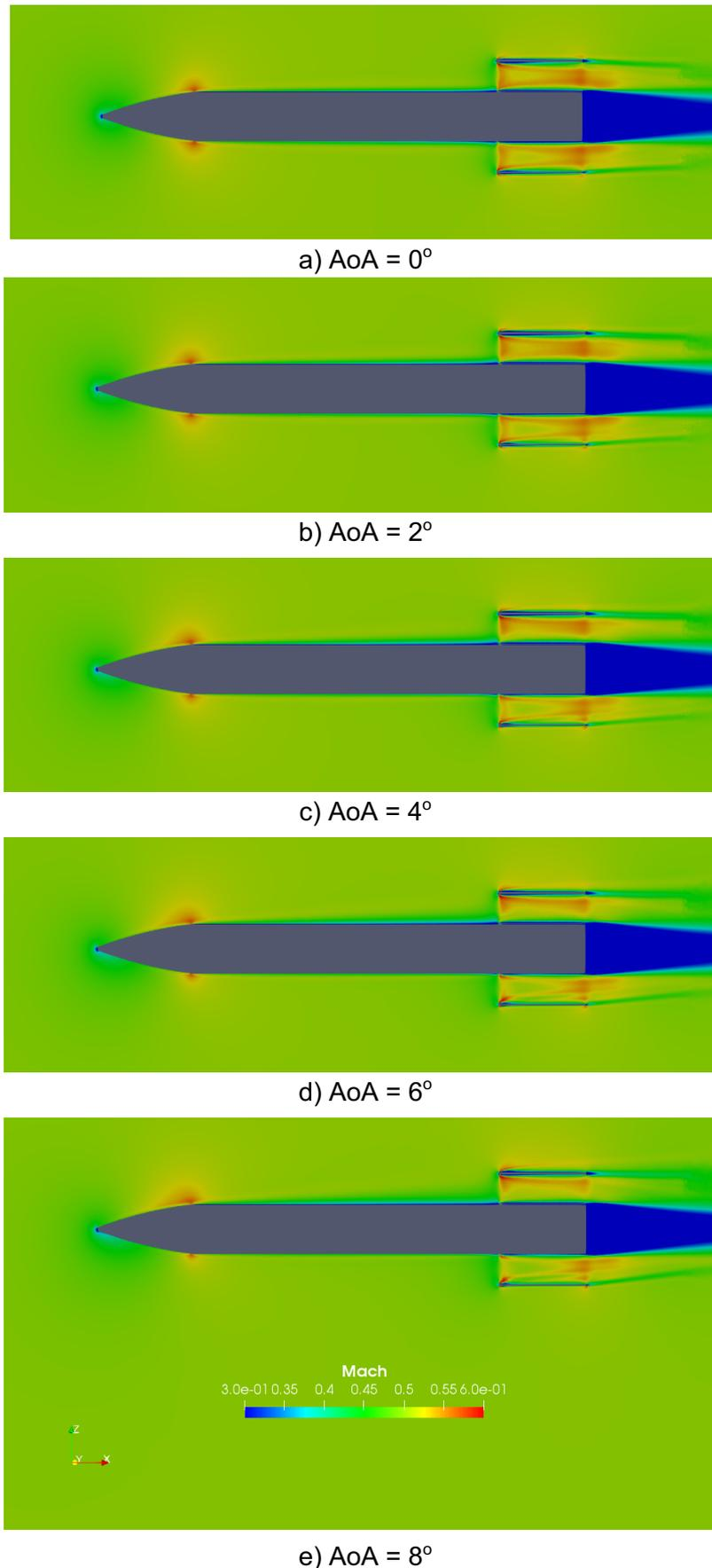
Figure 10: Mach contours at different angles of attack
