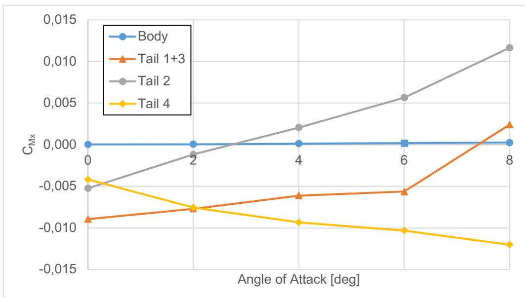
Figure 15. Roll Moment Contributions of Different Body Parts at Different Angles of Attack
