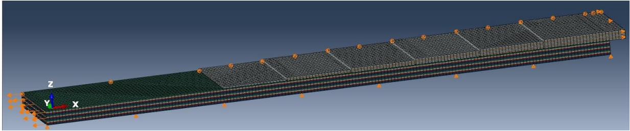
Figure 13 FEM for Stepped Double Lapped Repair Specimen
