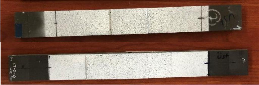
Figure 7 Repaired Composite Test Specimens
