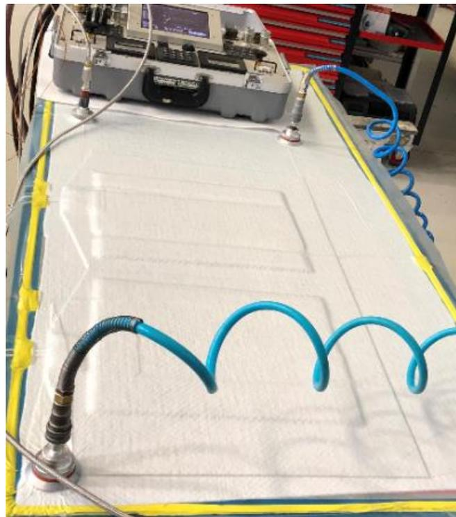
Figure 6 Curing of repair patch
