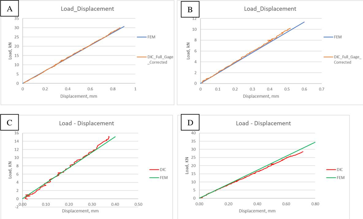
Figure 15 Load -Displacement Graphs from DIC system
