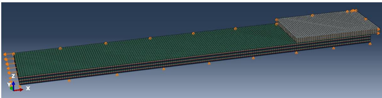
Figure 12 FEM for Uniform Double Lapped Repair Specimen
