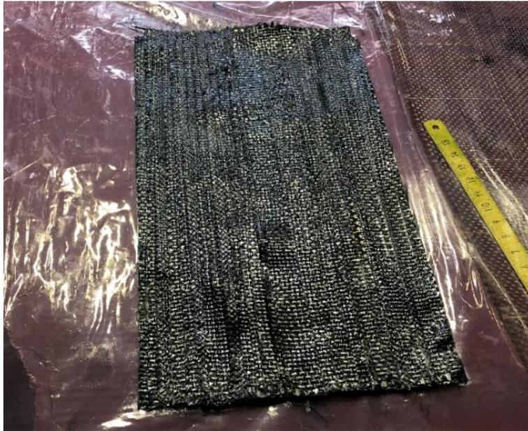
Figure 5 Repair patch before placing on the parent material
