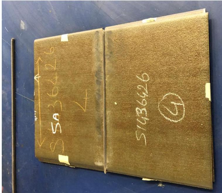
Figure 3 Parent flat plates and mandrel just before laying up the repair patch
