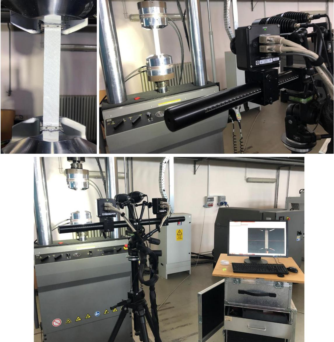
Figure 8 Tensile Testing Using DIC System
