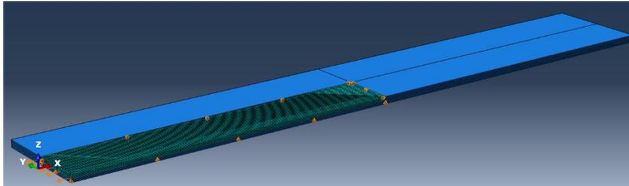
Figure 10 FEM for Plain Specimen of Repair Patch Material
