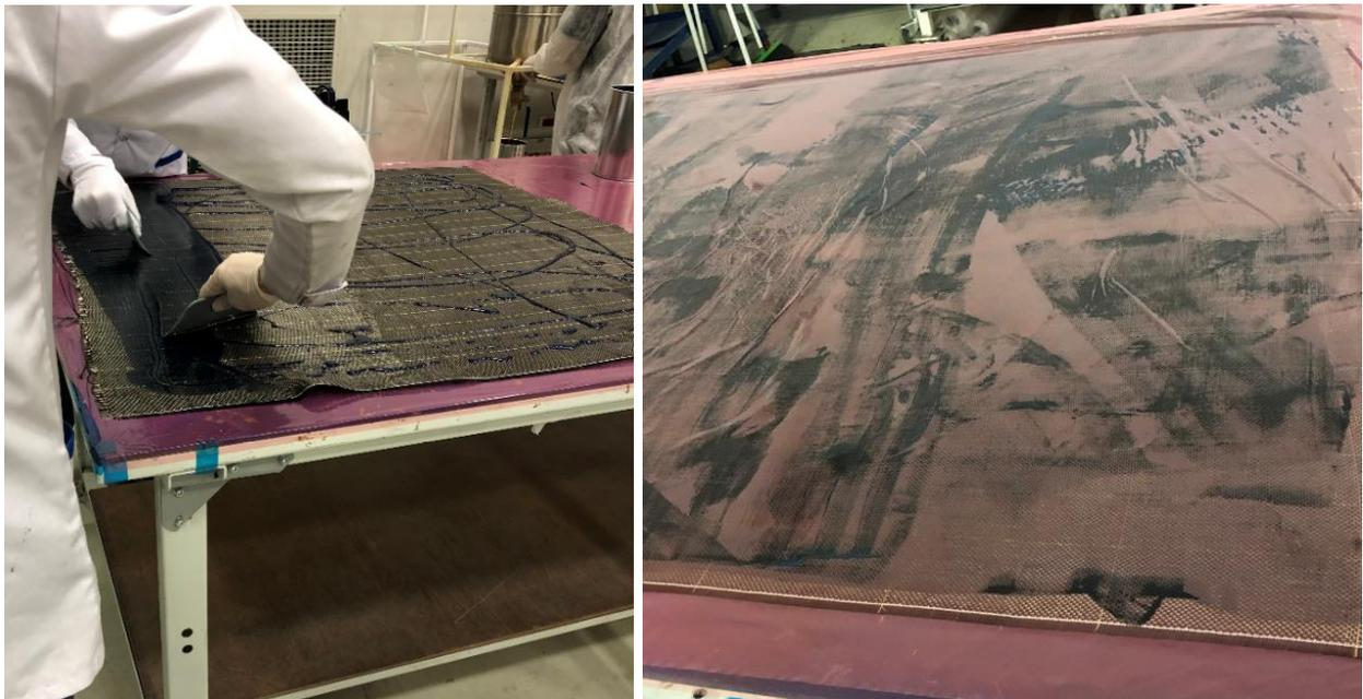
Figure 4 Wet lay up of dry fabric
