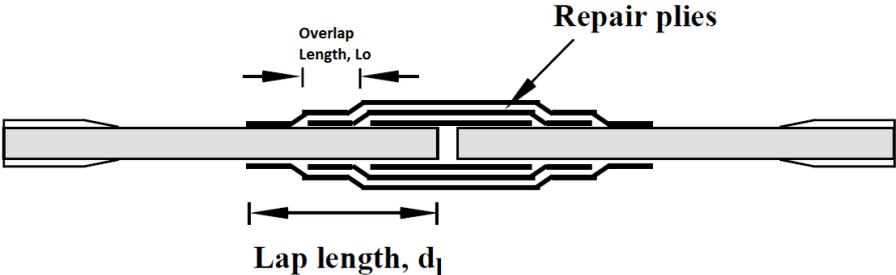
Figure 2: Stepped Double Lap Repair Tensile Test Specimen [Ahn, 2000]
