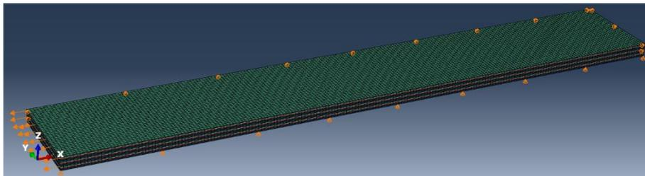
Figure 11 FEM for Plain Specimen of Parent Material
