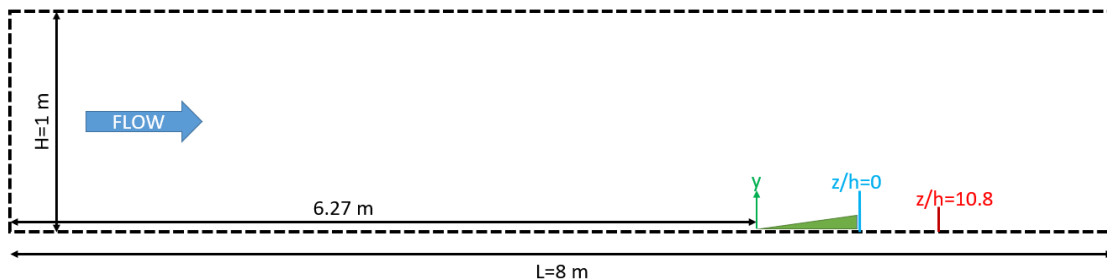
Figure 13: Schematic for the placement of MVG inside the tunnel [Akpolat et al., 2021]
