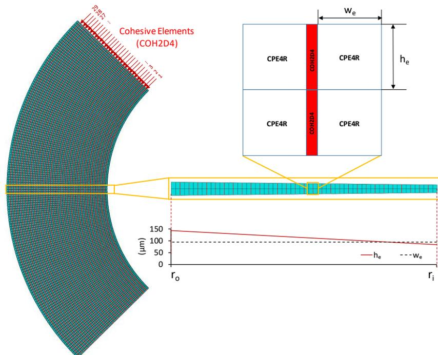
Figure 2: Mesh density at the curved region of the two-dimensional finite element model and details on interface modelling
