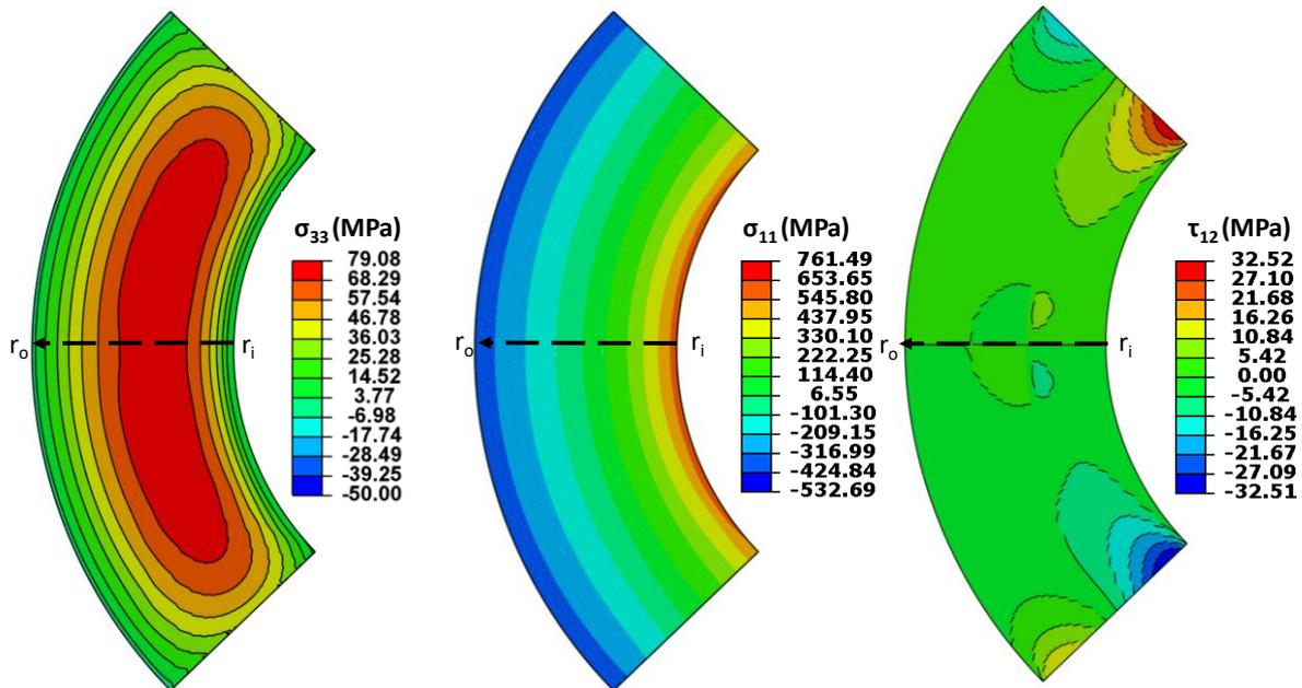
Figure 4: Radial, tangential and shear stress contours at the curved region 0.5  $\mu$ s before delamination initiation
