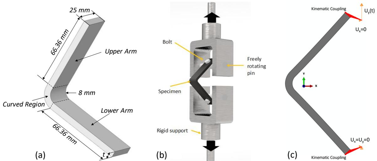
Figure 1: (a) Specimen geometry for the curved UD laminate, (b) Schematic of experimental configuration showing how the specimen is located in the fixture [ Tasdemir , 2019 ], (c) Boundary conditions in 2D finite element model
