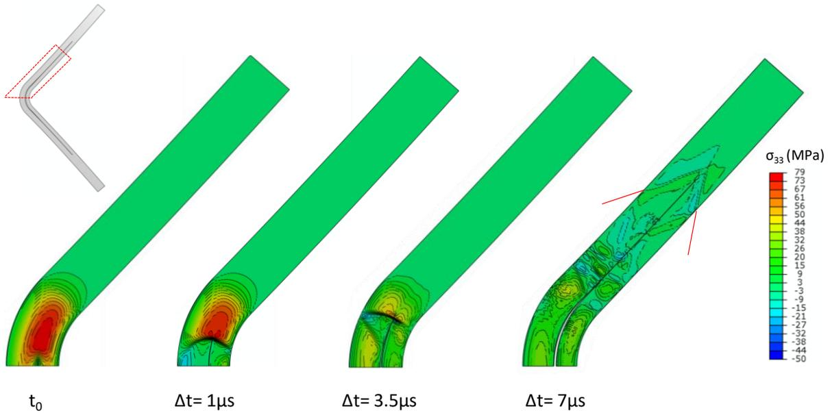
Figure 6: Stress distributions before and after delamination initiation
