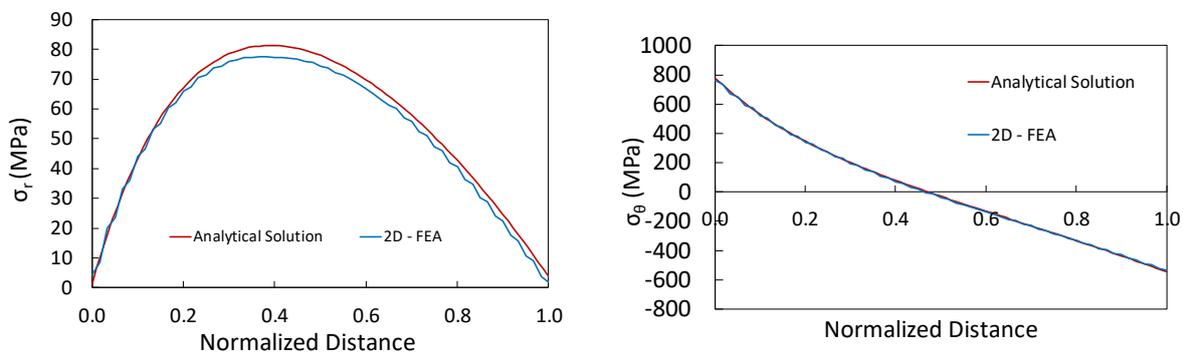
Figure 5: Comparison of 2D FEA and analytical solution for radial and tangential stresses along the defined path through the thickness at the mid-line of the curve.
