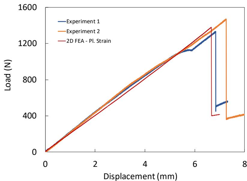
Figure 3: Load-displacement curves from 2D FEA and experiments of Tasdemir [ Tasdemir, 2018 ]
