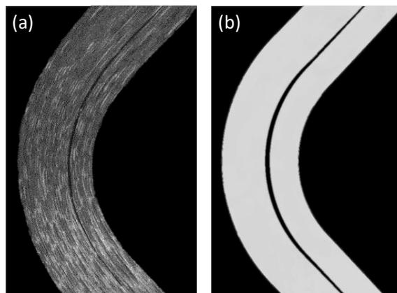
Figure 7: Delamination location on fully deformed specimen from (a) experiment [ Tasdemir, 2018 ] and (b) 2D finite element analysis
