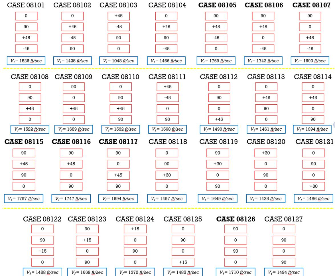
Figure 9: Flutter Results for 8-plyes E-Glass Fin at 27 different orientations
