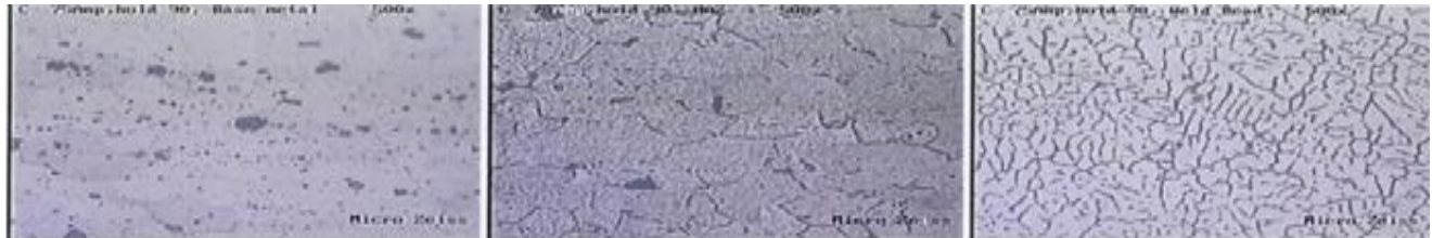
Figure 7 Micrographs showing the Microstructure of(BM,HAZ,FZ) 1.5 mm, 2024 Aluminum
