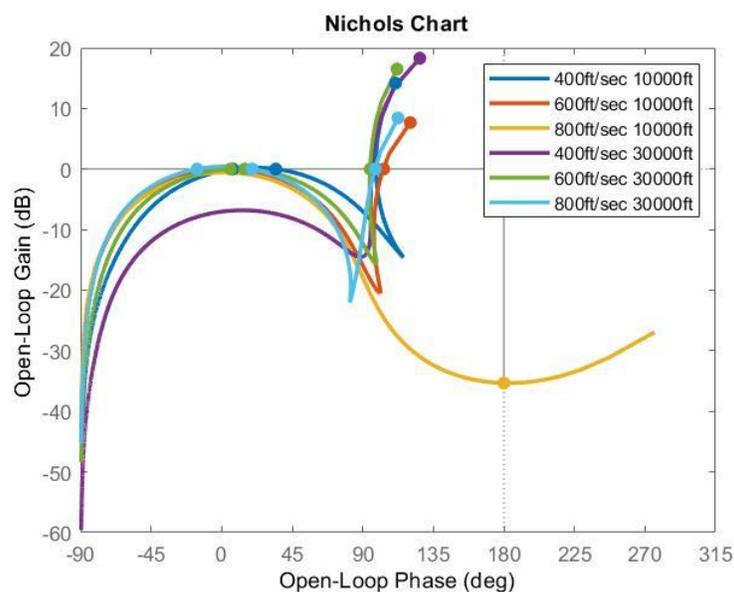
Figure 3: Nichols plot for the loop gain from rudder input
