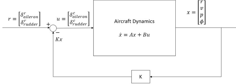
Figure 1: Stability augmentation system on lateral-directional axes
