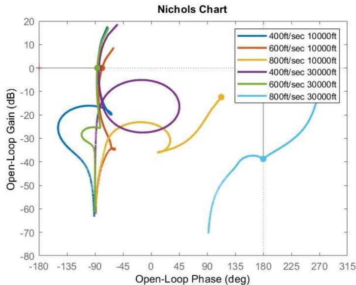
Figure 2: Nichols plot for the loop gain from aileron input
