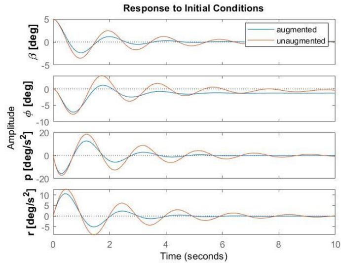
Figure 5: Initial time response of augmented aircraft
