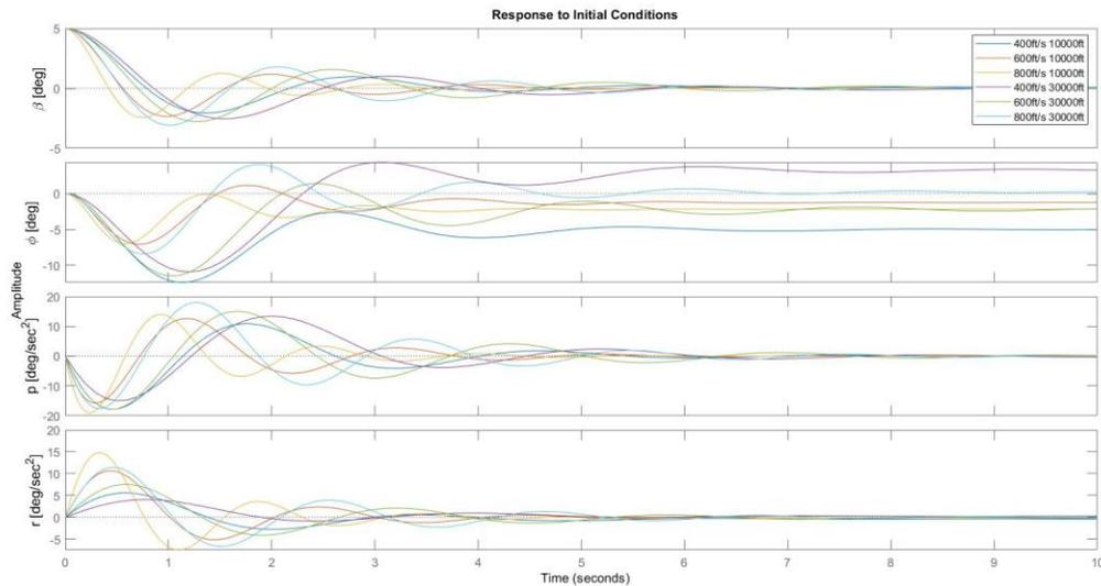
Figure 4: Initial time response of augmented aircraft
