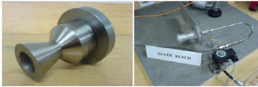
Figure 6: PRSS thruster (left) and static test bench (right) [Anis, 2008]
