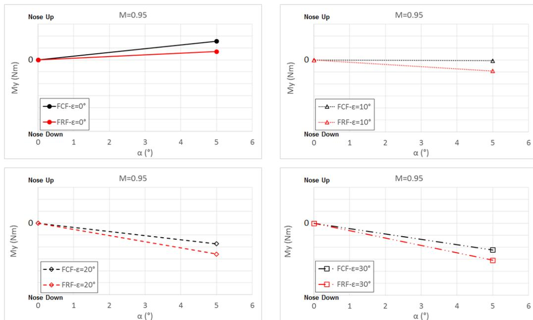
Figure 9: Pitching Moment vs  $\alpha$  curves @M=0.95 for Wing Angles ( $\epsilon = 0^\circ - 30^\circ$ )
