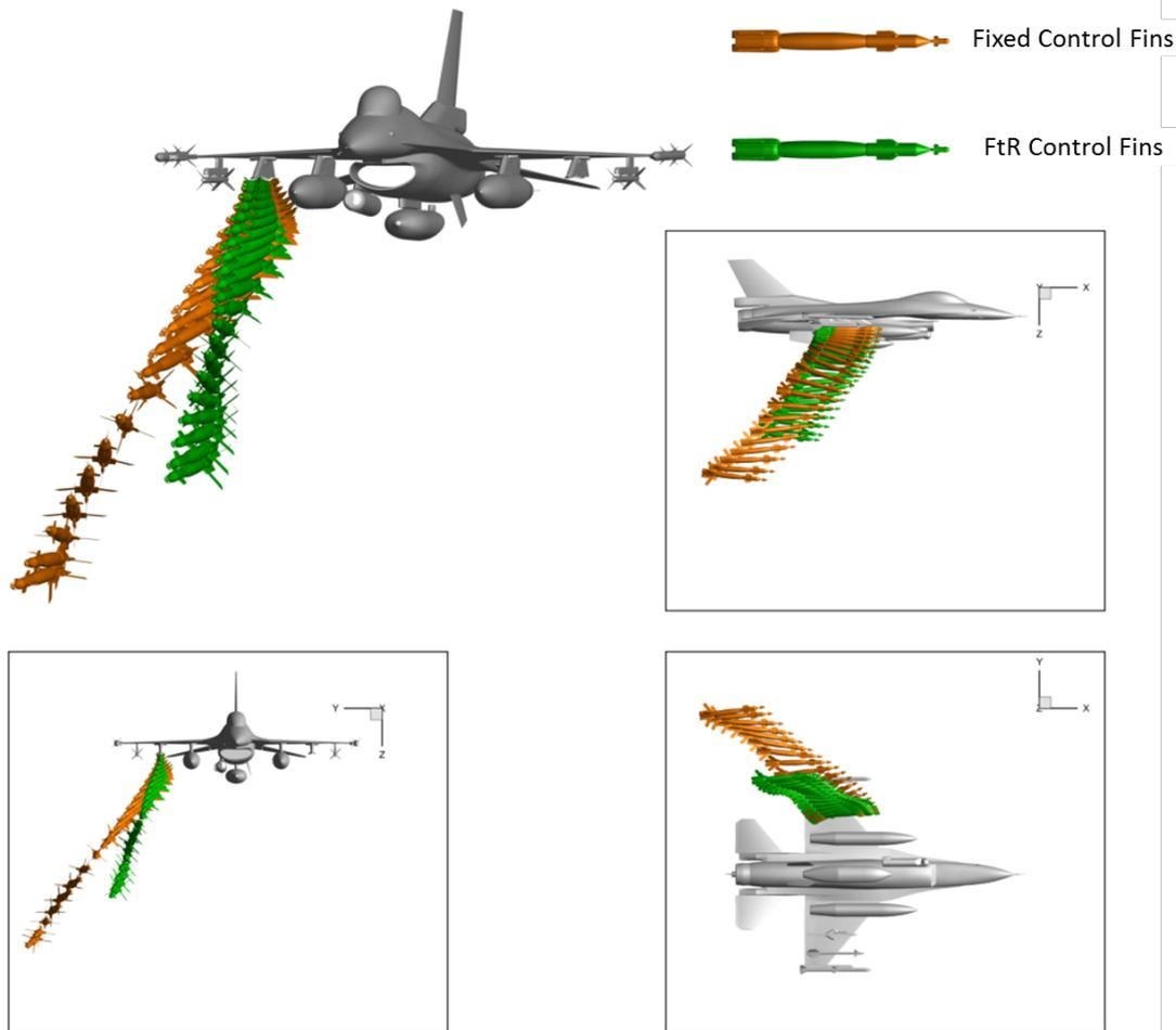
Figure 14: Deploying Wing FRF and FCF configuration
