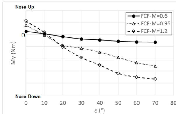
Figure 6: Fix Control Fins Configuration ( $\alpha = 5^\circ$ )
