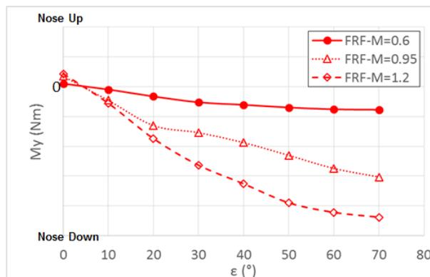
Figure 7: Free to Rotate Control Fins Configuration ( $\alpha = 5^\circ$ )
