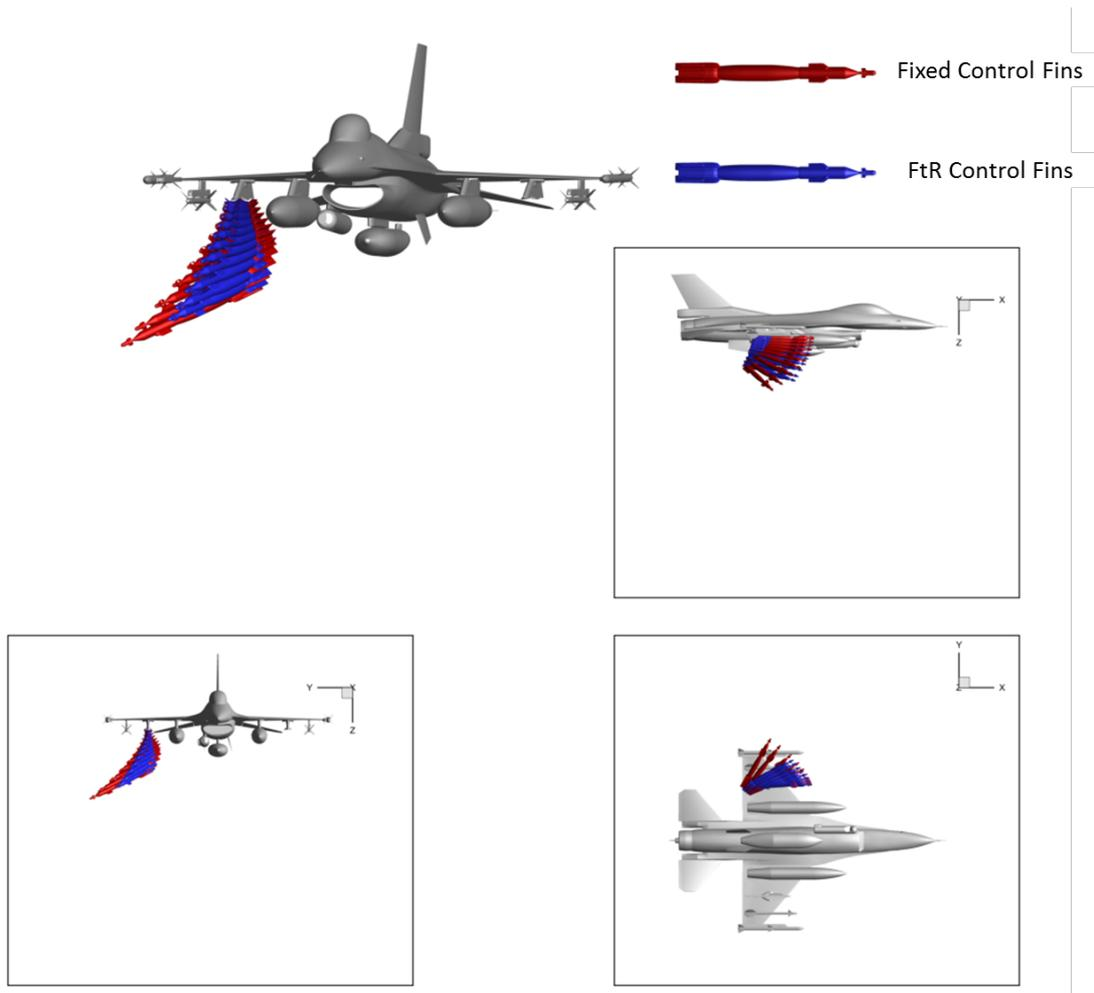
Figure 11: Stowed Wing FRF and FCF configuration
