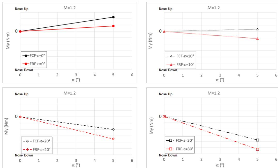
Figure 10: Pitching Moment vs  $\alpha$  curves @M=1.20 for Wing Angles ( $\epsilon = 0^\circ - 30^\circ$ )
