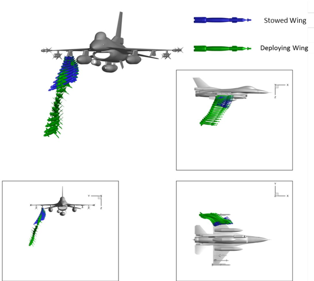
Figure 12: FRF Configuration wing effect
