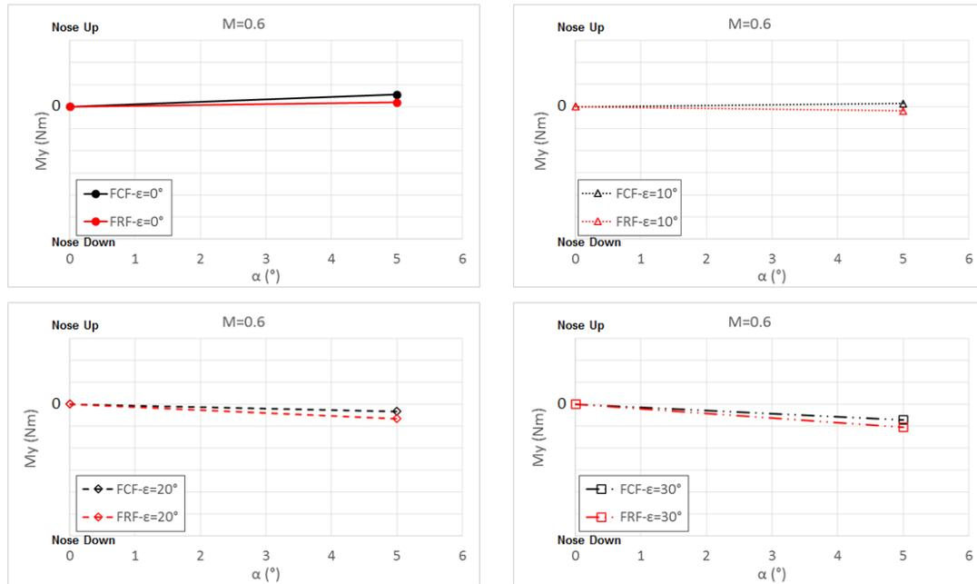
Figure 8: Pitching Moment vs  $\alpha$  curves @M=0.60 for Wing Angles ( $\epsilon = 0^\circ - 30^\circ$ )
