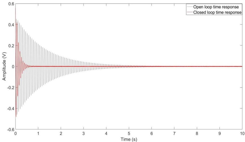
Figure 8: Experimental response of the smart beam: Free vibration case
