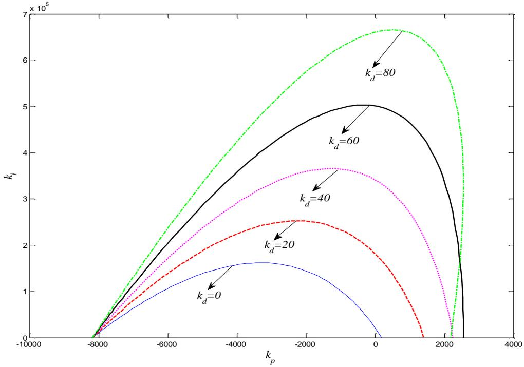
Figure 6: Regions of stable controller parameters according to derivative gain
