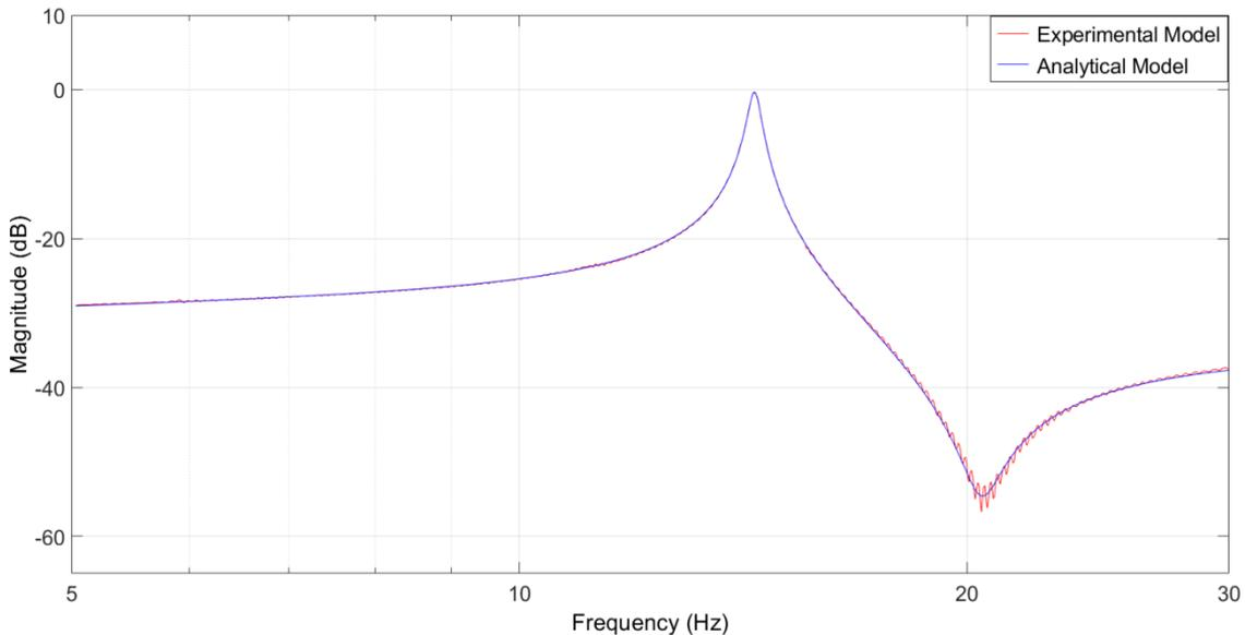
Figure 3: Frequency response of experimental and analytical models of smart beam
