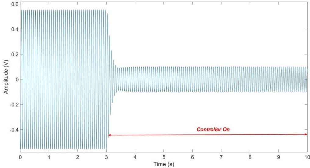
Figure 9: Experimental response of the smart beam: Forced vibration case at the first resonance frequency
