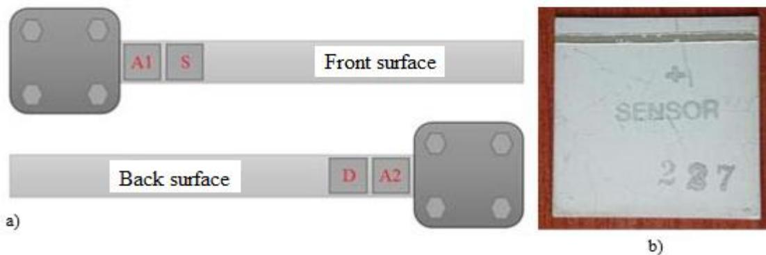
Figure 1: a) Labels of the PZT patches, b) PZT patch (BMP500) [Akin,2015]
