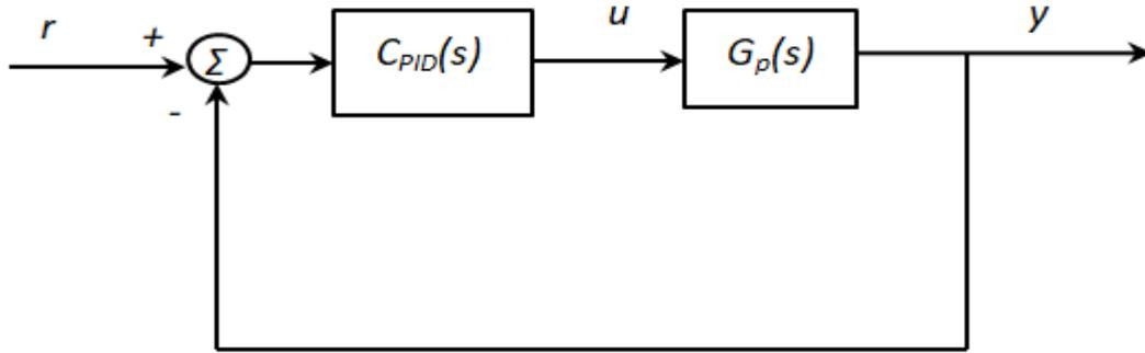
Figure 4: PID control system
