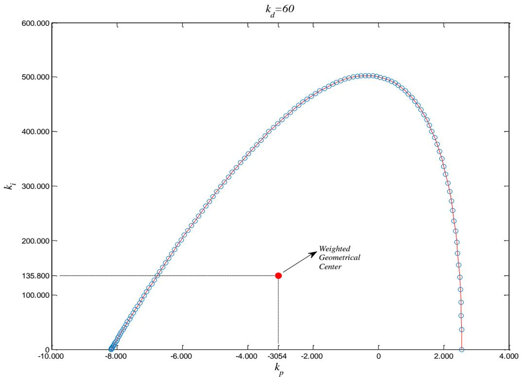
Figure 7:  $k_d = 60$  which makes it stable for the  $k_p$ - $k_i$  controller parameters region and its weighted geometrical center
