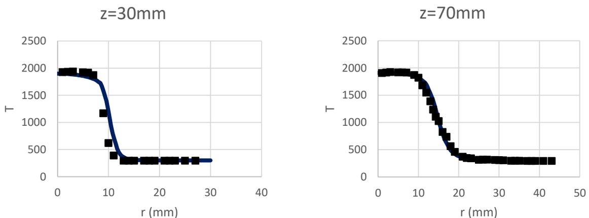
**Figure 3** The temperature profiles in SwB3 flame at  $z = 30\text{mm}$  (left) and  $z=70\text{ mm}$  (right). The dots: experimental measurements, solid line: the results calculated with the present solver.
