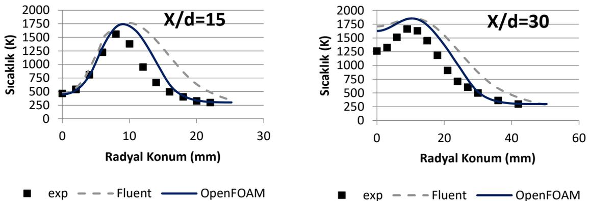
**Figure 2** The temperature profiles in Sandia D flame at  $x/d=15$  (left) and  $x/d=30$  (right). The dots: experimental measurements, solid line: the results calculated with the present solver, the dashed line: the results calculated with Fluent.
