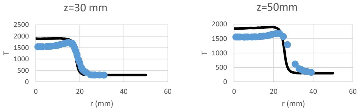
**Figure 5** The temperature profiles in SwB3 flame at  $z = 30\text{mm}$  (left) and  $z=50\text{ mm}$  (right). The dots: experimental measurements, solid line: the results calculated with the present solver.
