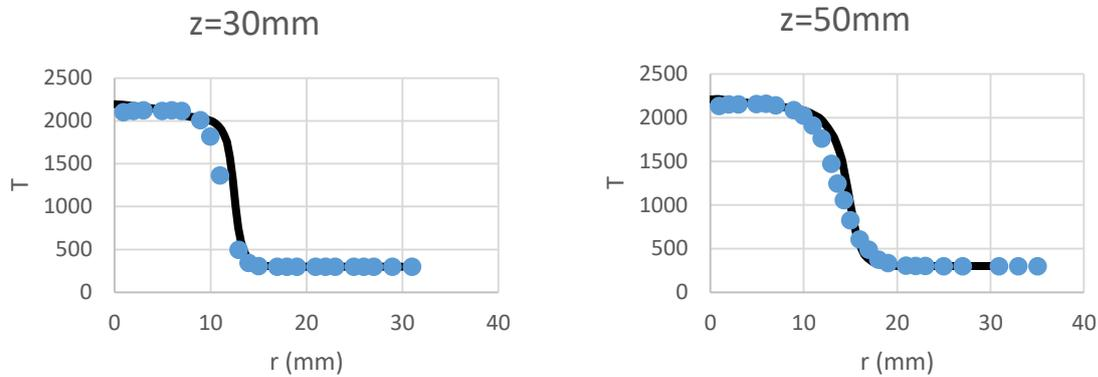
**Figure 4** The temperature profiles in SwB5 flame at  $z = 30\text{mm}$  (left) and  $z=50\text{ mm}$  (right). The dots: experimental measurements, solid line: the results calculated with the present solver.
