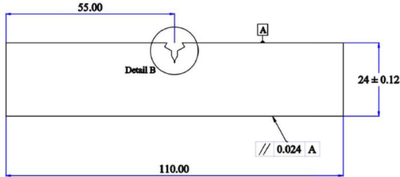
Figure 5. Drawing of single edge crack tension specimens (SET)
