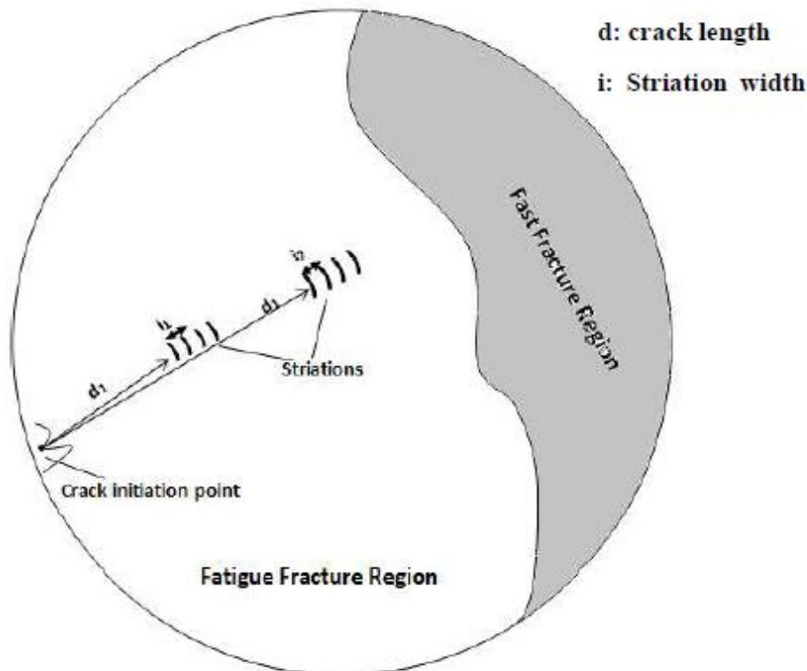
Figure 4. Striation width measurement method
