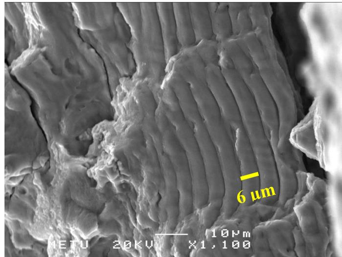
Figure 8. SEM image of striation width
