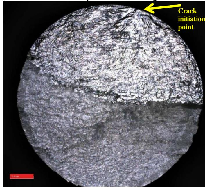
Figure 6. Fracture surface of failed test specimen specimen
