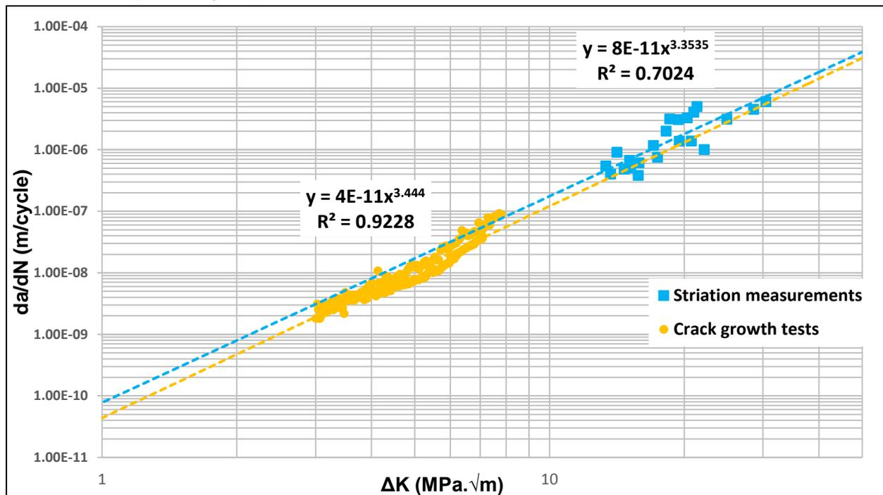
Figure 10. da/dN curves of 7050 T7451 Aluminum alloy
