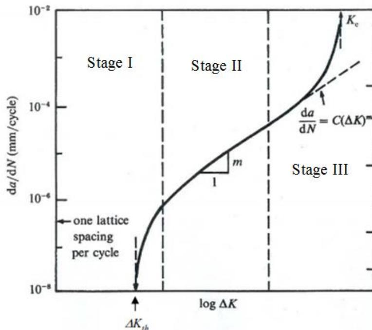
Figure 1. Crack Growth stages
