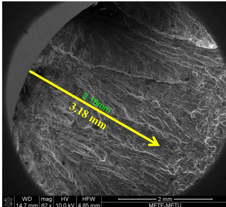
Figure 7. SEM image of distance away form crack initiation points
