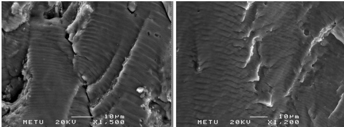
Figure 9 Striations from fracture surfaces
