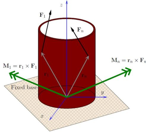
Figures-6 A CC with external forces represented by torsors.
