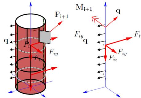
Figure-4 A real CC and its idealized model for the 3-D analysis
