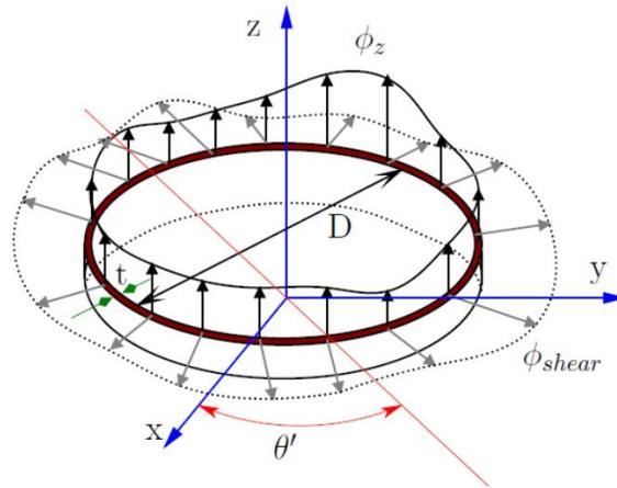
Figure-6 Representation of axial flux distribution at the base of a CC
