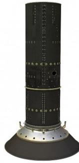
Figure-1 The typical Central cylinder (CC)
