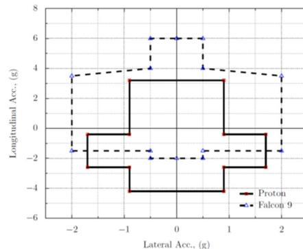
Figure-2 The quasi-static load envelopes for the Proton and Falcon 9 launchers
