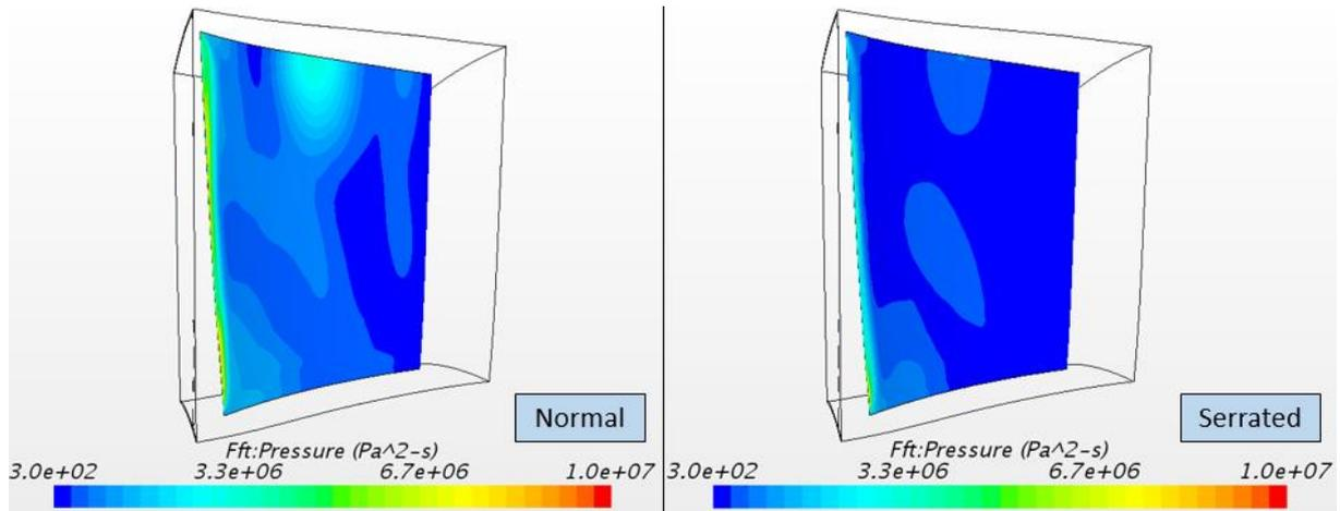
Figure 23: Pressure fluctuation energy on stator surface
