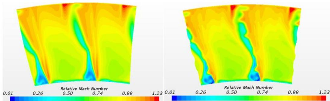
Figure 9: Original rotor (left) and serrated rotor conf.1 (right) relative Mach number contours
