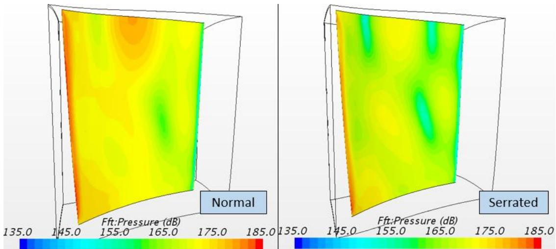
Figure 24: Noise source on stator surface [dB]
