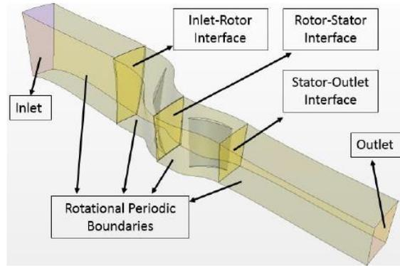
Figure 5: CFD domain and boundary conditions of compressor stage
