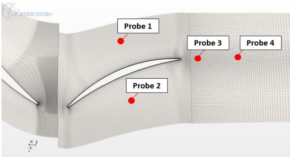
Figure 14: Pressure probes near stator blade
