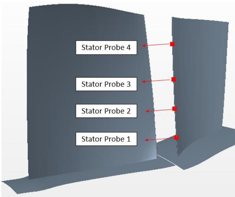
Figure 19: Stator surface pressure probes
