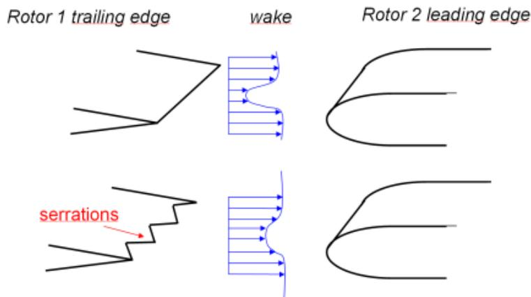
Figure 2: Serrations effect on rotor wake.
