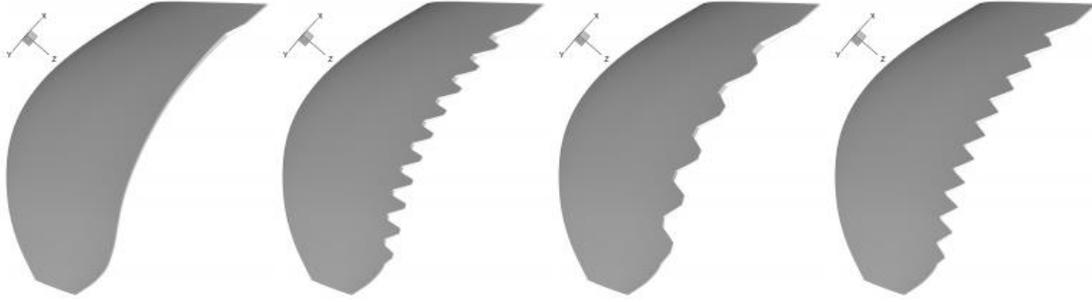
Figure 3: Different serrated trailing edge configurations [Weckmuller and Guerin, 2012]
