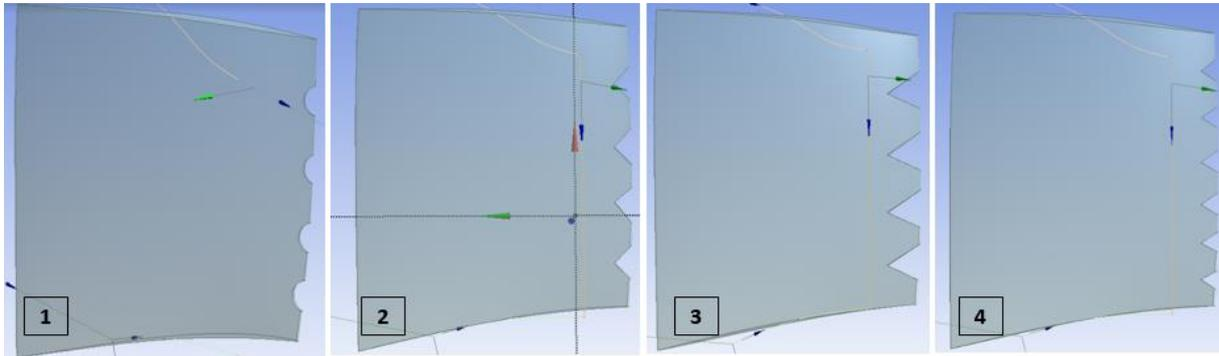
Figure 4: Different rotor serrated trailing edge configurations
