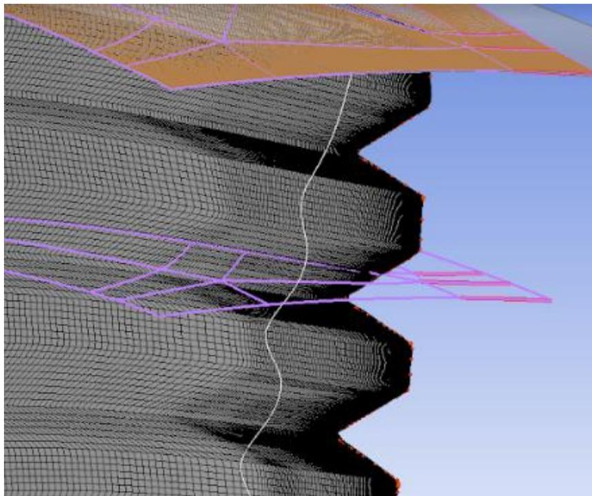
Figure 7: Serrated trailing edge rotor domain mesh
