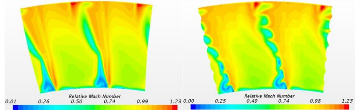
Figure 12: Original rotor (left) and serrated rotor conf.4(right) relative Mach number contours
