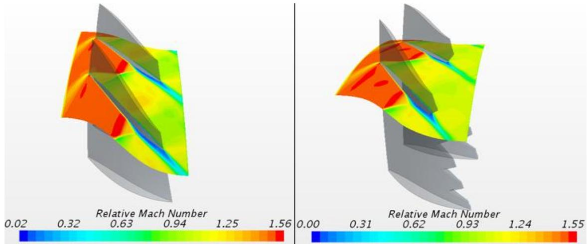
Figure 13: Original rotor (left) and serrated rotor conf.3(right) relative Mach number contours at 75% span
