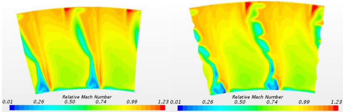
Figure 10: Original rotor (left) and serrated rotor conf.2 (right) relative Mach number contours
