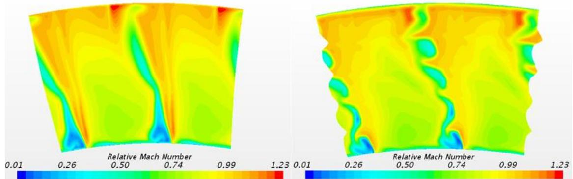
Figure 11: Original rotor (left) and serrated rotor conf.3(right) relative Mach number contours
