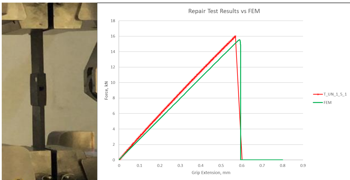
Figure 11: Abaqus Uniform Repair Model Load-Displacement Diagram vs Test Results
