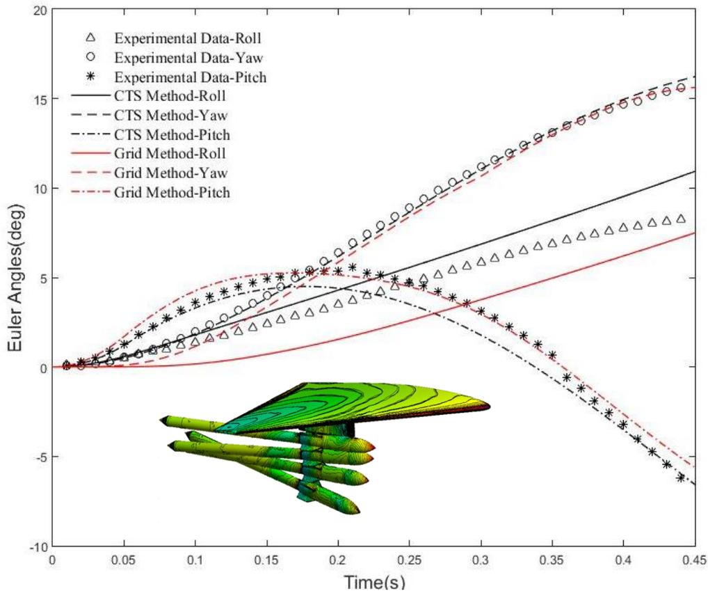
Figure 19: Comparison of estimated angular displacements for both techniques with experimental study
