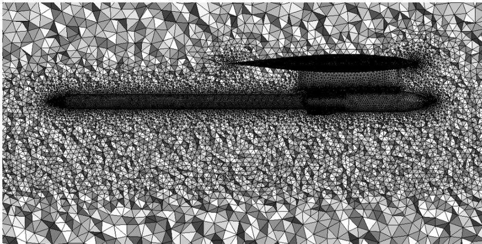
Figure 3: Section view of computational grid elements of whole domain
