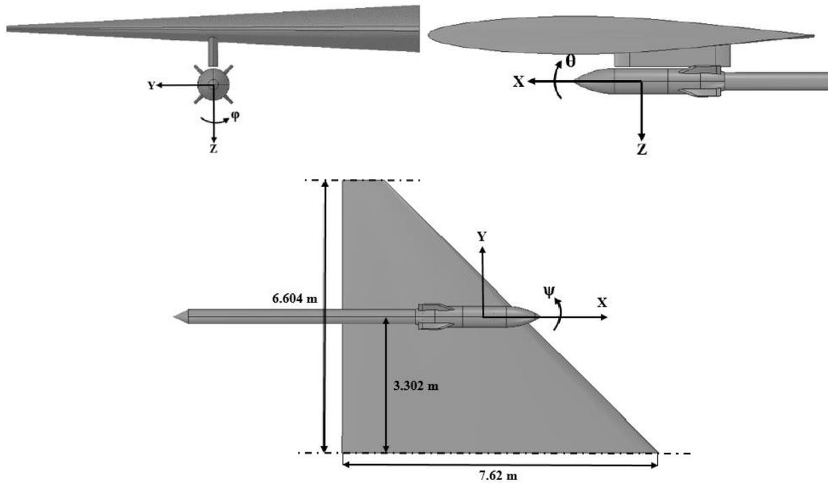
Figure 2: Geometrical details and coordinate system convention of computational model
