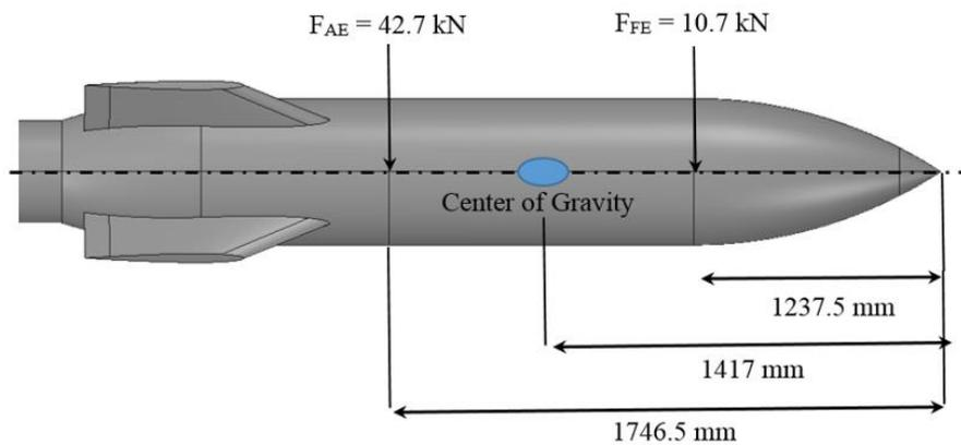
Figure 12: Location of ejector forces acting on the store
