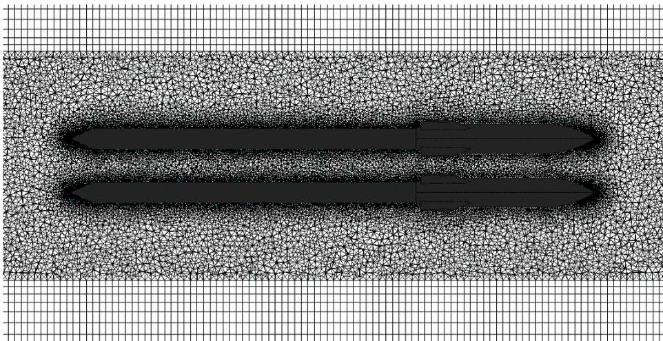
Figure 7: Computational grid domain of two store alone configuration
