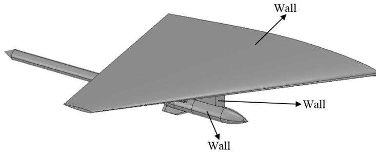
Figure 9: Boundary conditions of wing, pylon, store and sting
