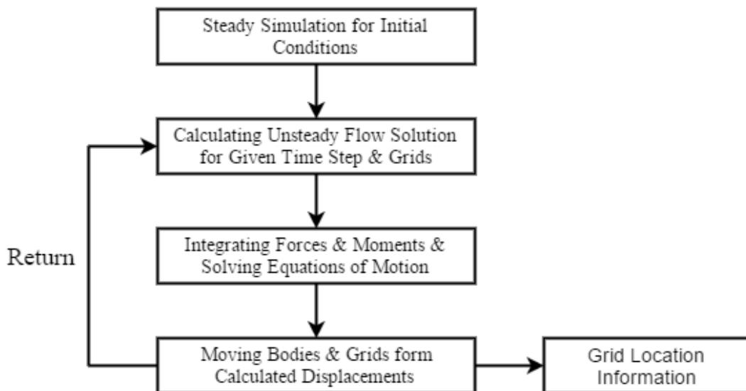
Figure 11: Flow chart of moving grid algorithm
