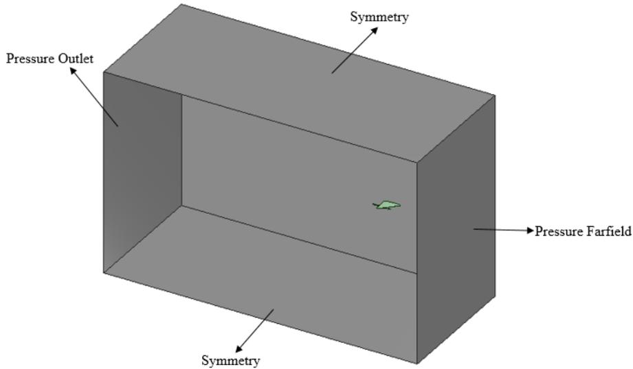
Figure 10: Boundary conditions of computational domain
