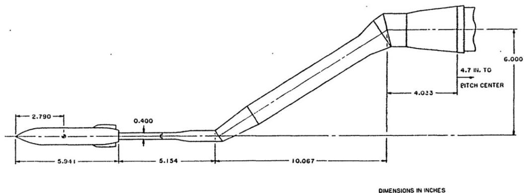
Figure 1: Wind tunnel setup dimensions
