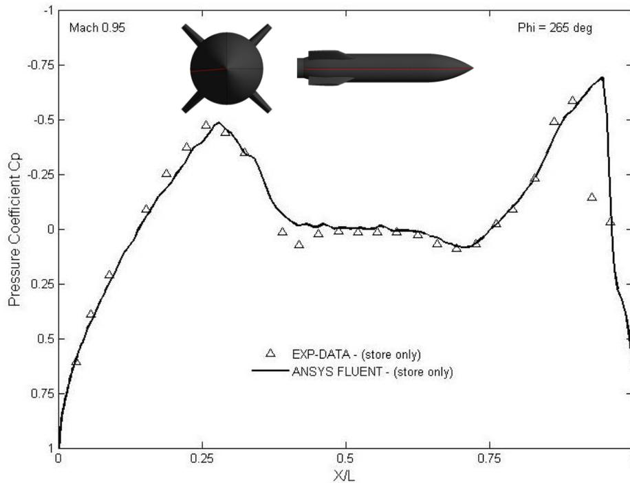
Figure 6: Pressure coefficient distribution of store-alone configuration
