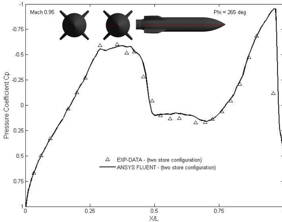
Figure 8: Pressure coefficient distribution for two store alone configuration
