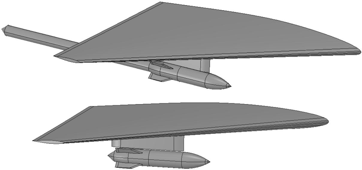
Figure 15: Isometric view of wing-pylon-smooth ended store configuration
