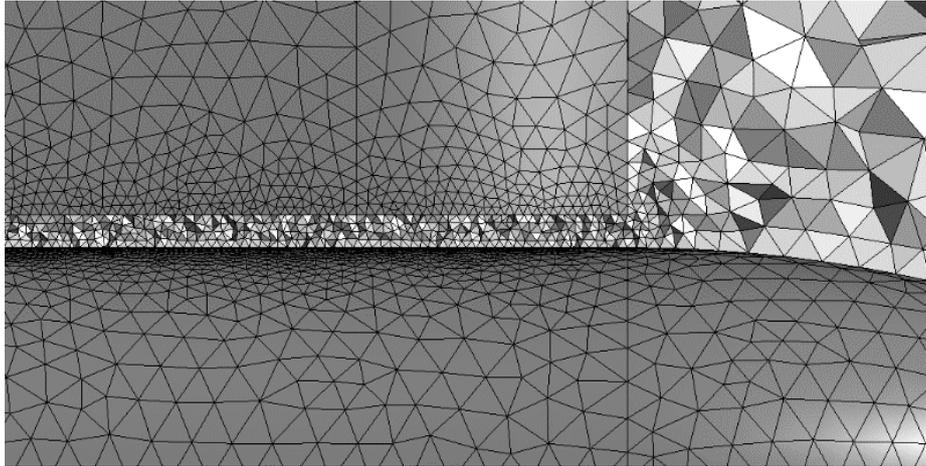
Figure 4: Detailed view of gap between pylon and store
