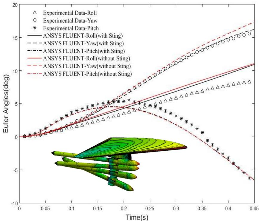
Figure 17: Comparison of estimated angular displacements for two store geometric configuration with experimental study
