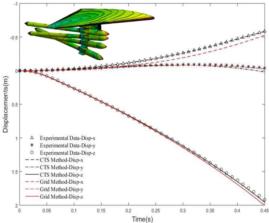
Figure 18: Comparison of estimated linear displacements for both techniques with experimental study
