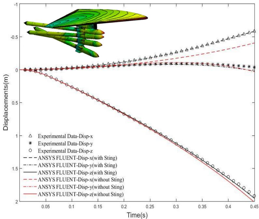
Figure 16: Comparison of estimated linear displacements for two store geometric configuration with experimental study
