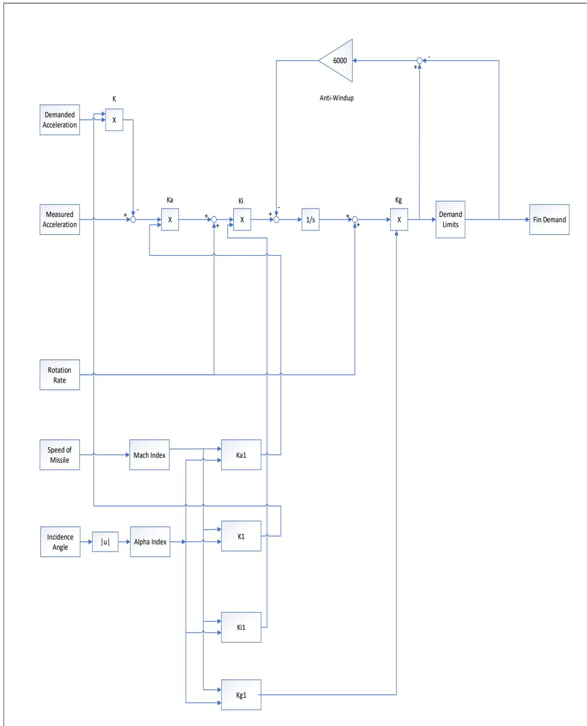
Figure 4: The proposed adaptive autopilot system.
