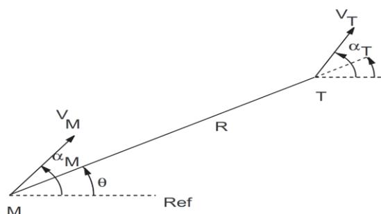
Figure 1: Engagement geometry of missile distant from the target.
