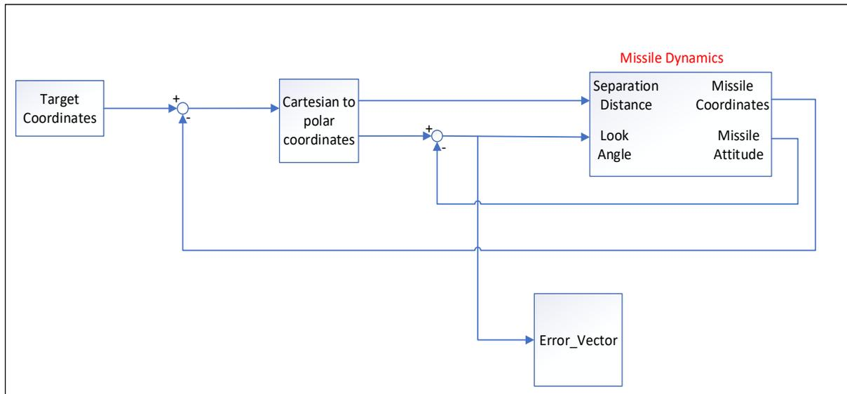
Figure 3: The feedback control system of the missile.
