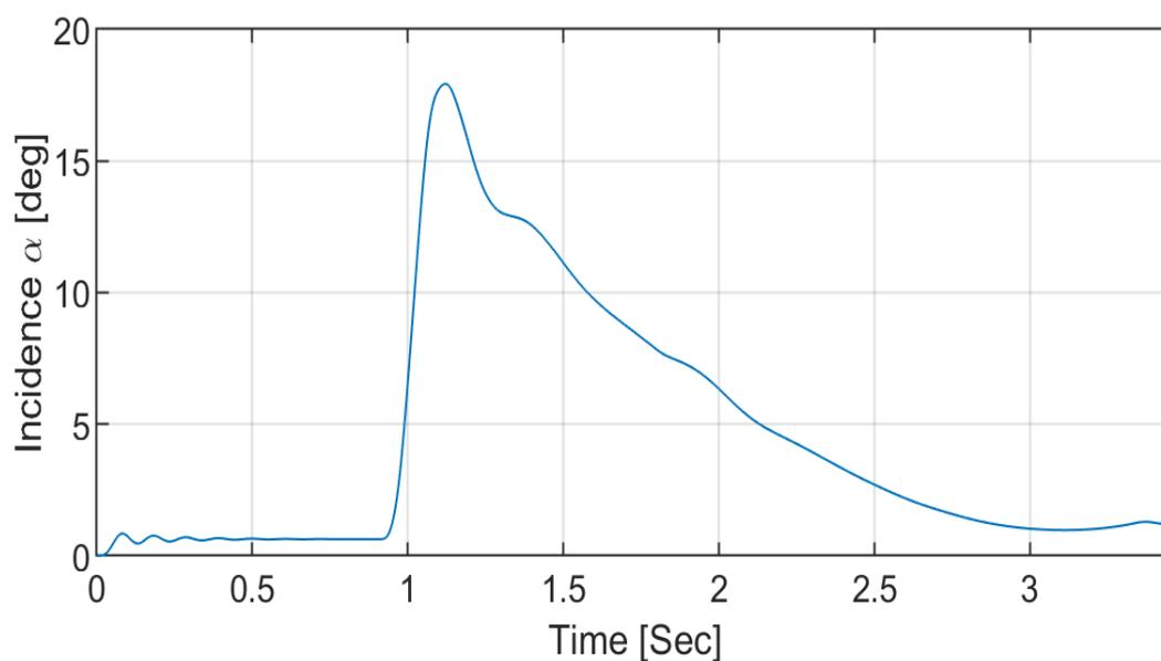
Figure 8: Incidence angle of the missile during flight.
