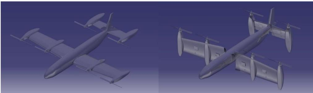
Figure 1: VTOL Tilt-Wing Aircraft in Different Flight Conditions
