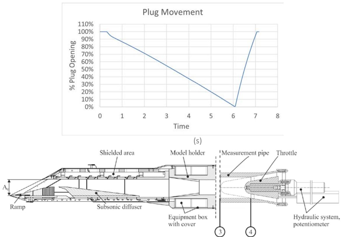
Figure 3: Plug movement (left), back area control scheme (right)
