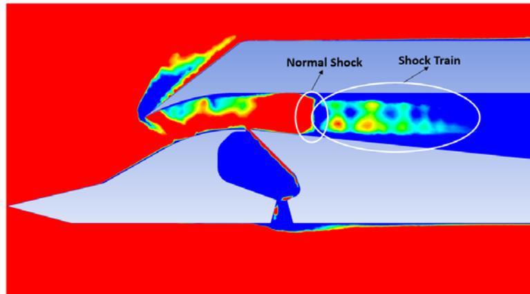
Figure 8: Terminal Normal Shock and Shock Train for NP3
