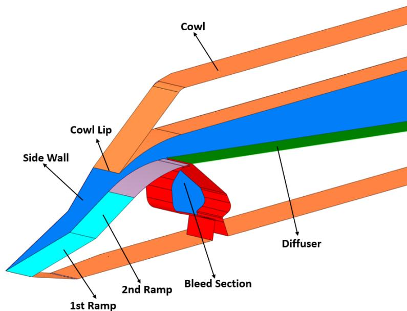
Figure 3: Elements of Air-Intake Model
