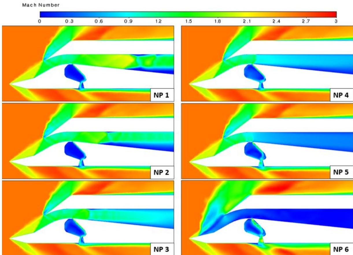
Figure 7: Variation of Terminal Shock Position with Nozzle Parameter
