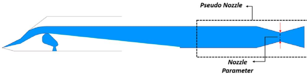
Figure 6: Pseudo Nozzle for the CFD Simulations and Nozzle Parameter for Back Pressure Adjustment
