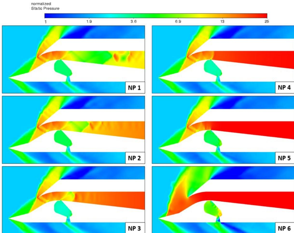
Figure 9: Static Pressure contours at different nozzle parameters (logarithmic scale)
