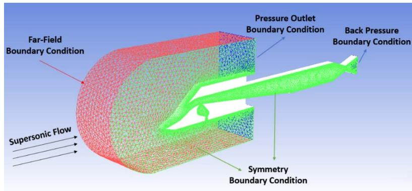
Figure 4: Boundary Conditions of the Simulation Model.
