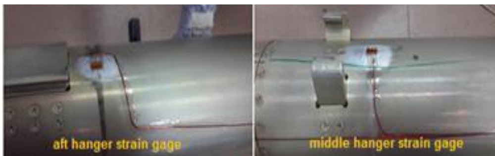
Figure 3: Locations of rosette strain gages on the DMS
