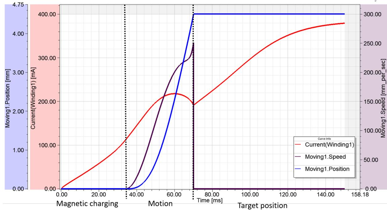
Figure 2: Behavior of typical solenoid
