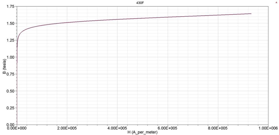
Figure 3: B-H curve of 430F steel[Brauer , 2014]
