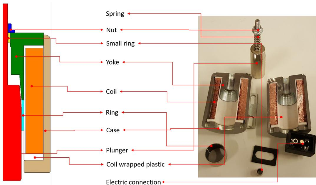
Figure 1: The cross section model of solenoid actuator and off-the-shelf solenoid.
