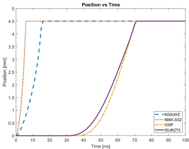
Figure 9: Analyses with 430F, NMX-S52, N30UHZ, and 50JN270 materials' position versus time graph
