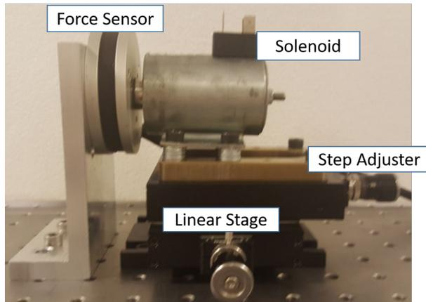
Figure 4: Spring constant experiment setup
