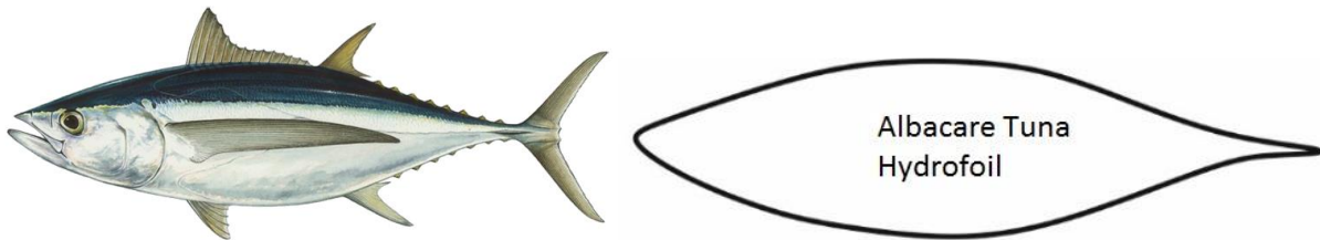
Figure 2: Albacore Tuna (left, image courtesy of Diane Rome Peebles at igfa.org) and the hydrofoil generated from the image (right)
