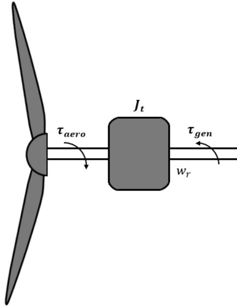
**Figure 4:** Wind Turbine Model Dynamics with One Mass
