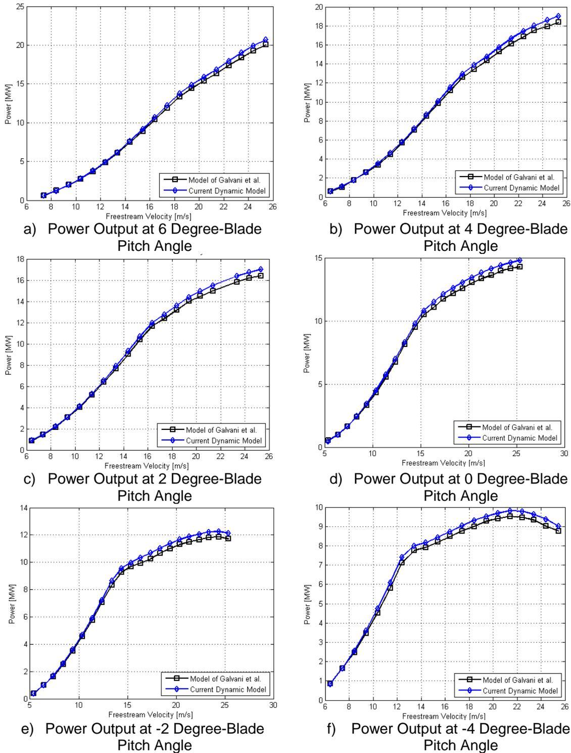
**Figure 5: Power Outputs of 5 MW Turbine at Various Pitch Angles**
