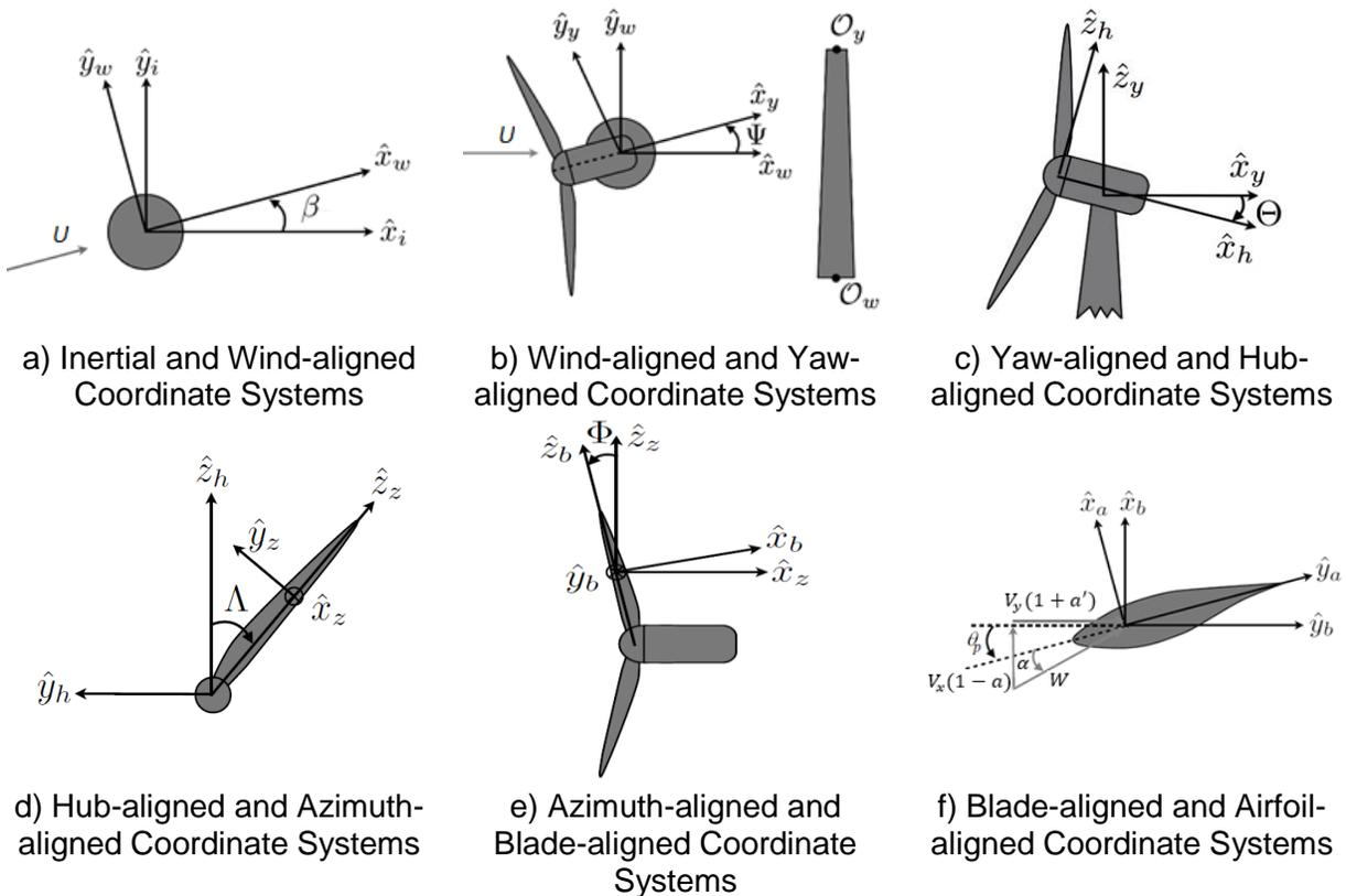
**Figure 3:** Wind Turbine Coordinate Systems [Ning, 2013]
