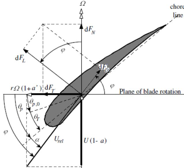
**Figure 2:** HAWT Blade Geometry [Manwell et al., 2002]
