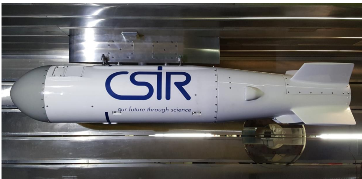
Figure 4: Inundu pod in the CSIR's transonic wind-tunnel for tests of its RAT
