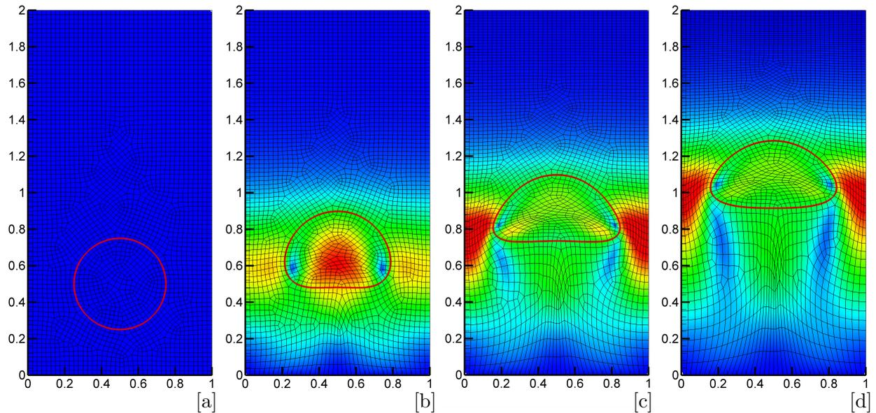
Figure 1: Mesh deformation on mesh M1 at time levels  $t=0$  [a],  $t=1$  [b],  $t=2$  [c] and  $t=3$  [d] with velocity magnitude contours.
