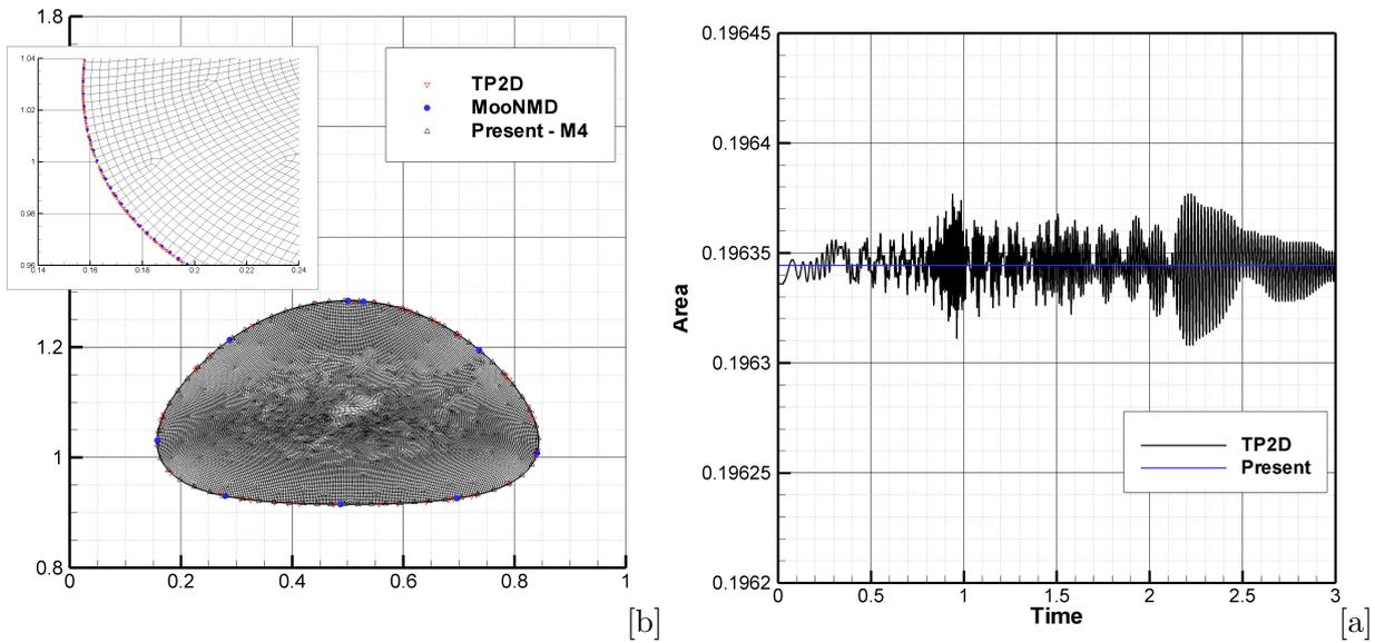
Figure 2: Comparison of bubble shapes on mesh M4 with TP2D (red) and MooNMD (blue) at  $t=3$  [a] and the comparison of the bubble area time variation with the result of TP2D [b].
