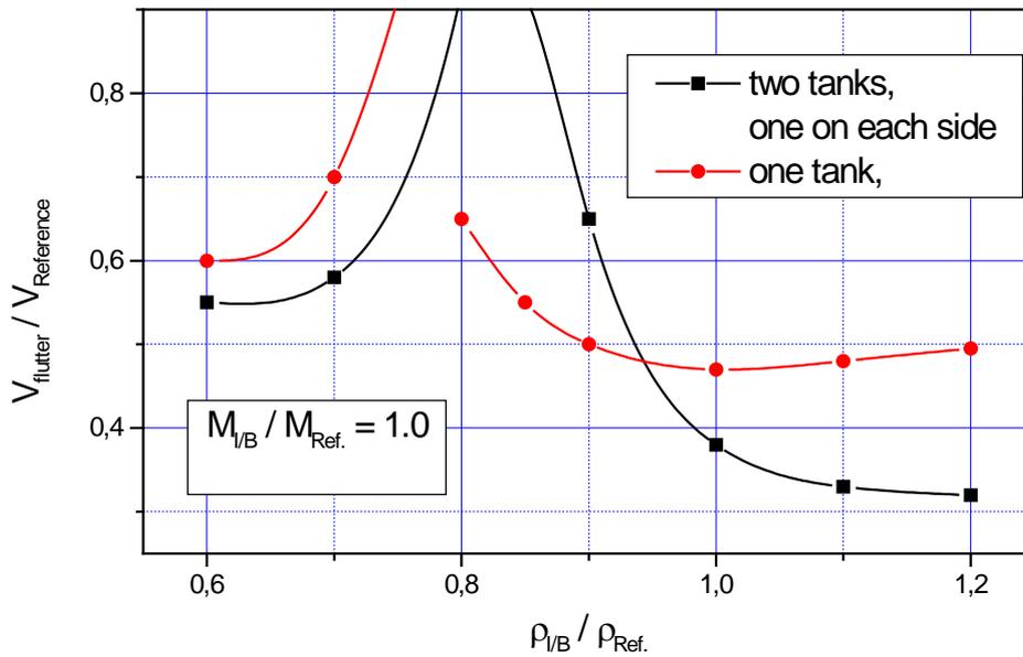
**Fig. 8: Flutter speed versus symmetric and asymmetric carriage, with radius of gyration variation**
