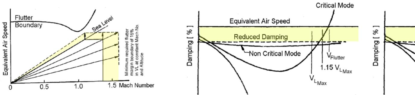
**Fig. 3: Graphical Representation of the Flutter Requirement MIL-A-8870**
