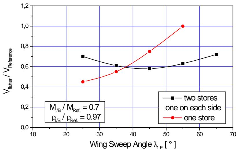
**Fig. 9: Flutter speed versus wing sweep angle symmetric and asymmetric carriage**
