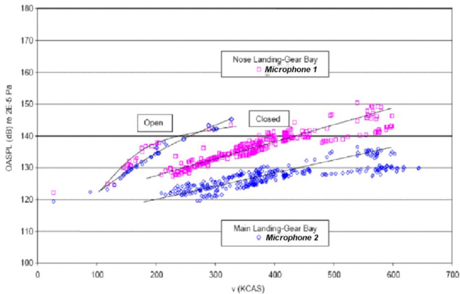
**Fig. 6: OASPL in opened and closed nose and main undercarriage bays in relation to velocity**
