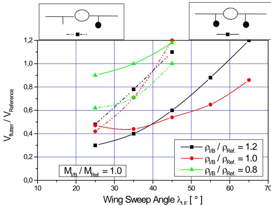
Fig. 10: Flutter speed versus wing sweep angle radius of gyration variation
