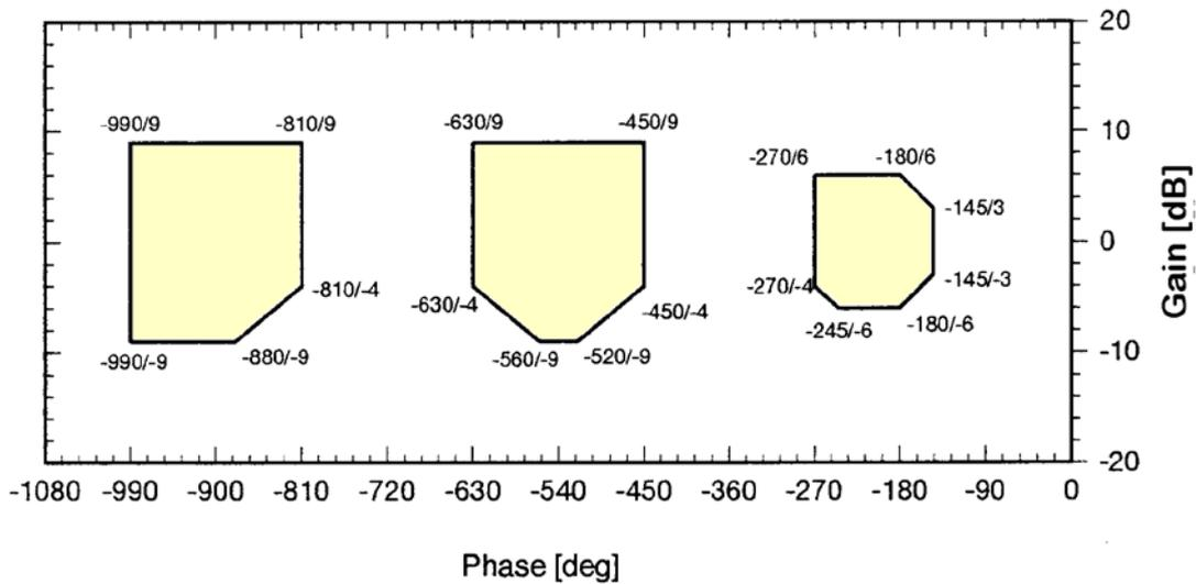
**Fig. 4: MIL-F-09490 Stability Margin Criteria for Open Loop Frequency Response Function**
