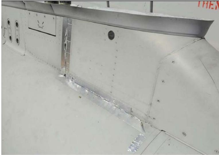
**Fig. 5: Cracks between tank and pylon and on integrated pylon panels (tried to repair by tape)**
