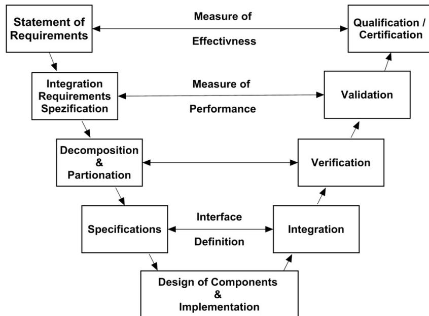
Fig. 2: V-Diagram for system integration process
