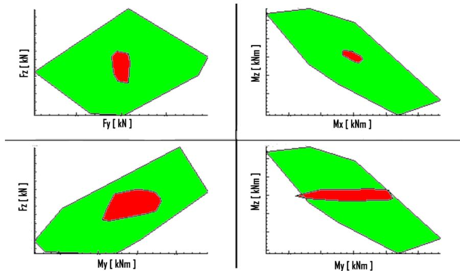
Fig. 7: Load Envelopes at pylon interface
