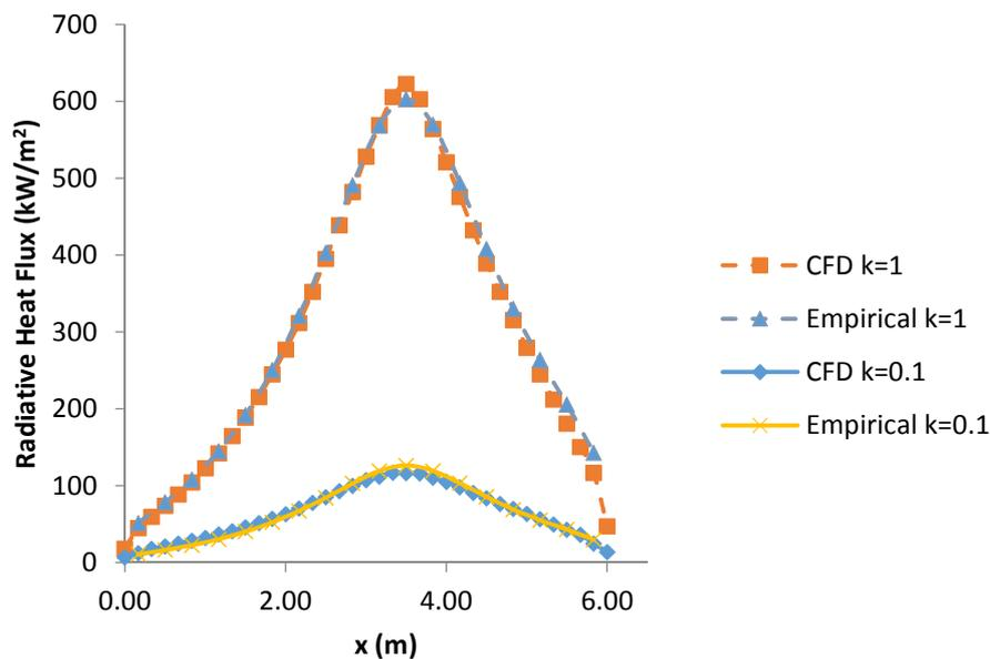
Figure 6: CFD and empirical calculation (by using view factor) comparison
