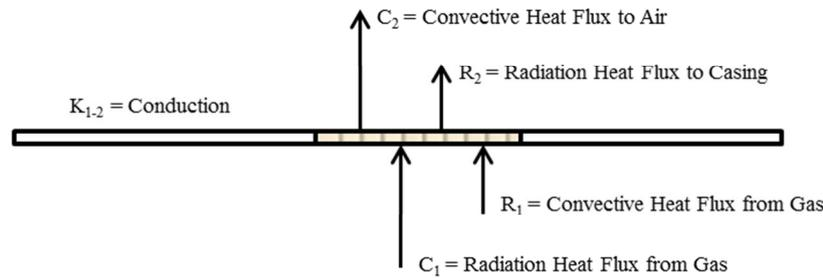
Figure 1: Basic heat transfer process in combustor liner
