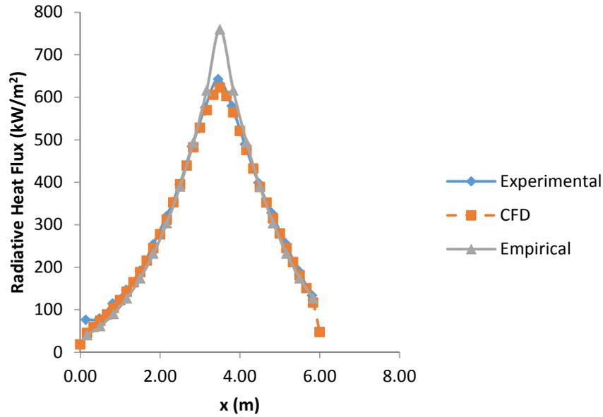
Figure 3: CFD and empirical calculation comparison for  $k=1 \text{ m}^{-1}$
