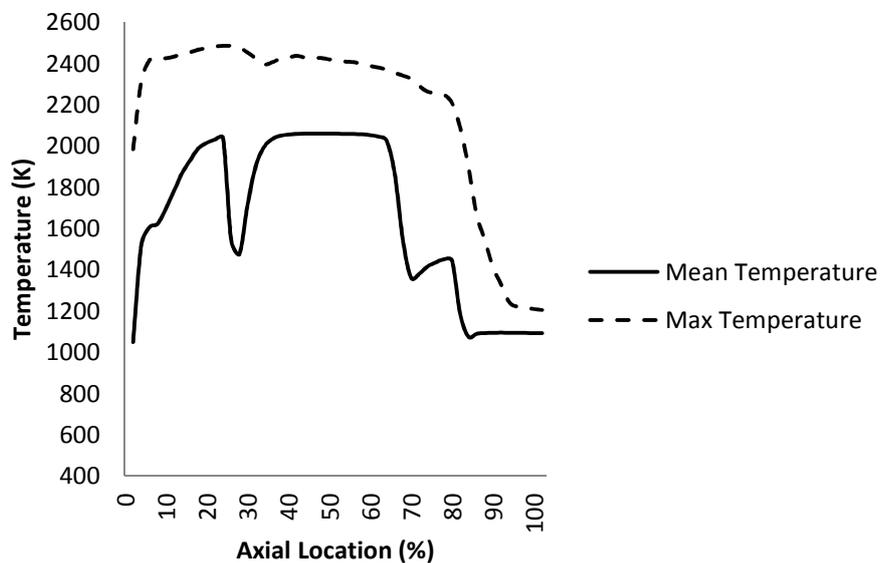
Figure 8: Mean and Maximum Gas Temperatures in the Flame Tube
