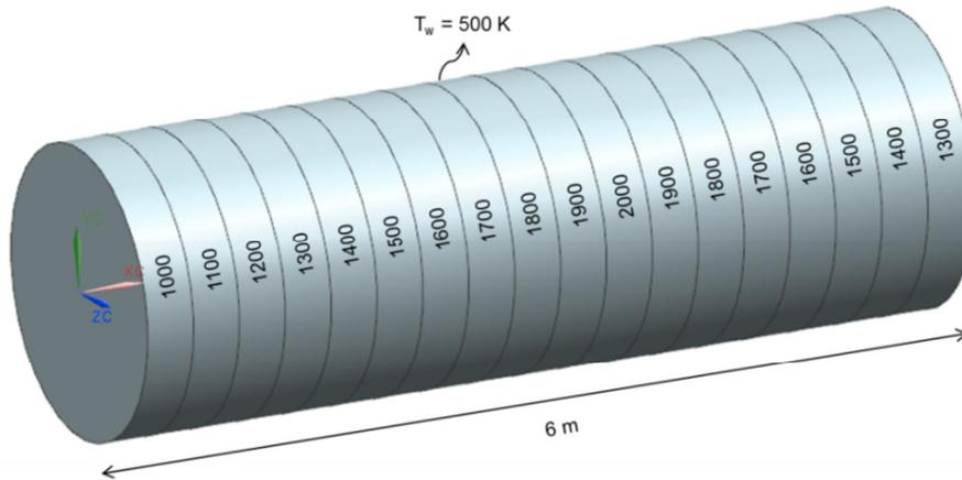
Figure 2: Case 1 (Cylinder geometry and gas temperature distribution)
