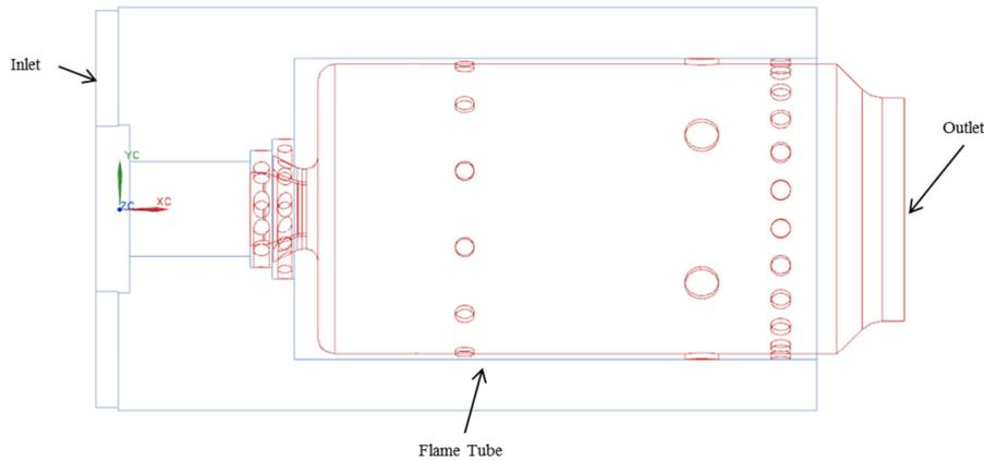
Figure 7: CFD Boundary Conditions
