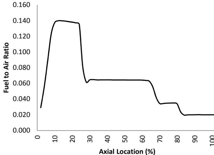
Figure 9: Fuel to Air Ratio Change through the Flame Tube
