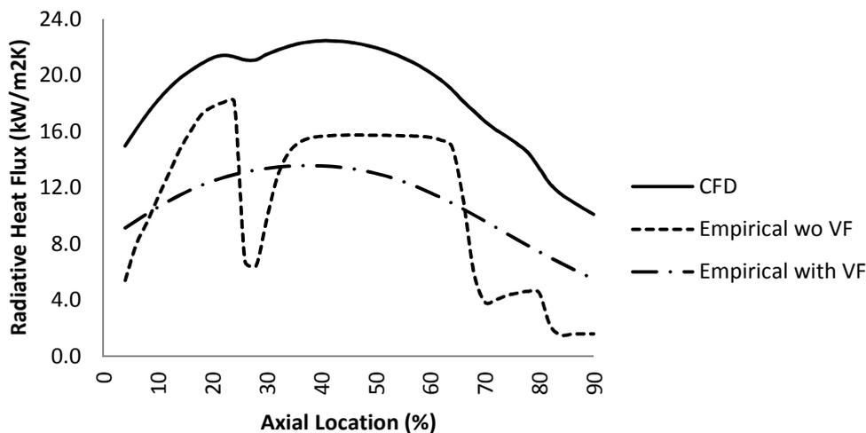
Figure 10: Axial Radiation Heat Flux Change Based on Mean Gas Temperatures
