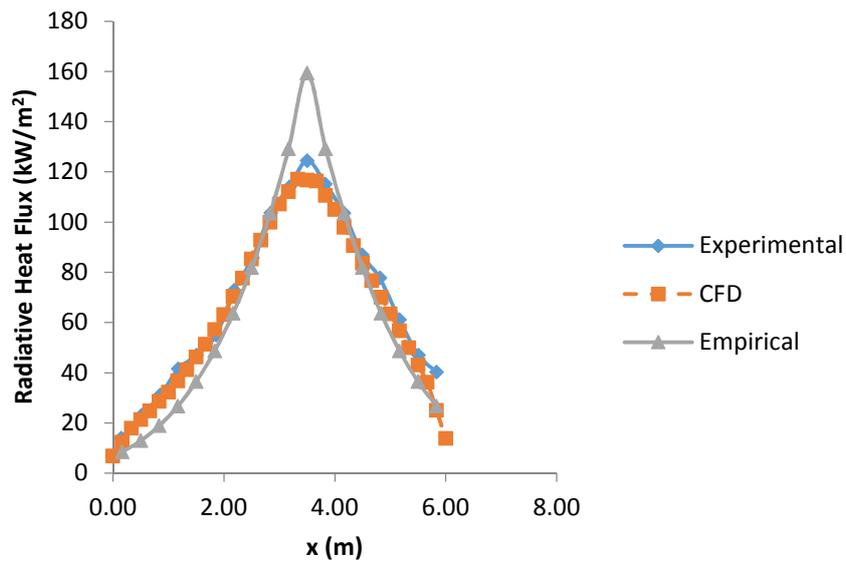
Figure 4: CFD and empirical calculation comparison for  $k=0.1 \text{ m}^{-1}$
