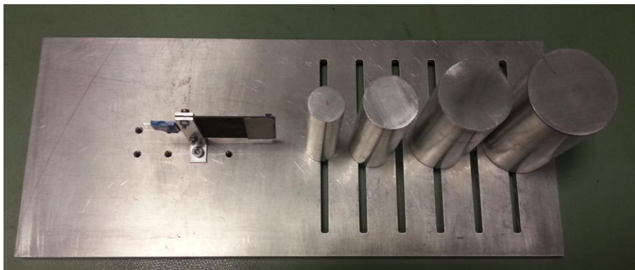
Figure 4: Manufactured Vortex Energy Harvester and Bluff Bodies
