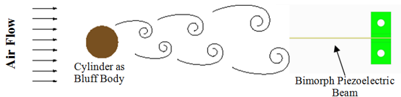
Figure 1: Vortex Energy Harvester with Cylinder and Plate as a Bluff Body
