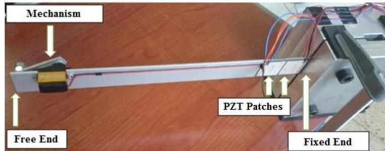
Figure 1: Smart Beam [Akin, O. & Sahin, M., 2015]
