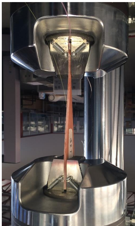
Figure 3: S2T under 20^\circ Angle of Twist
