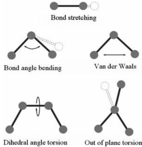
Figure 2: Deformation types of C bonds [Tserpes,2005]
