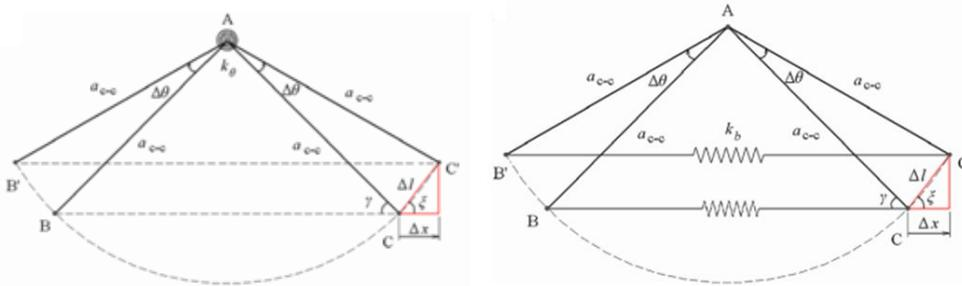
Figure 4: Torsional spring to linear spring stiffness evaluation [Giannopolus,2007]
