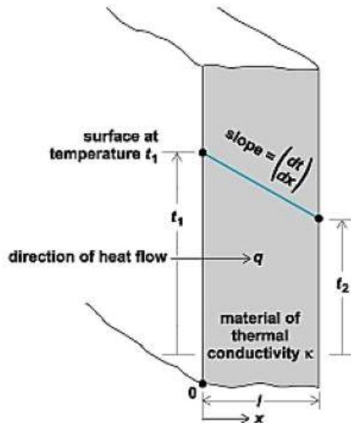
Figure 4: One-dimensional conduction heat transfer [<http://www.accessscience.com>, 2013]
