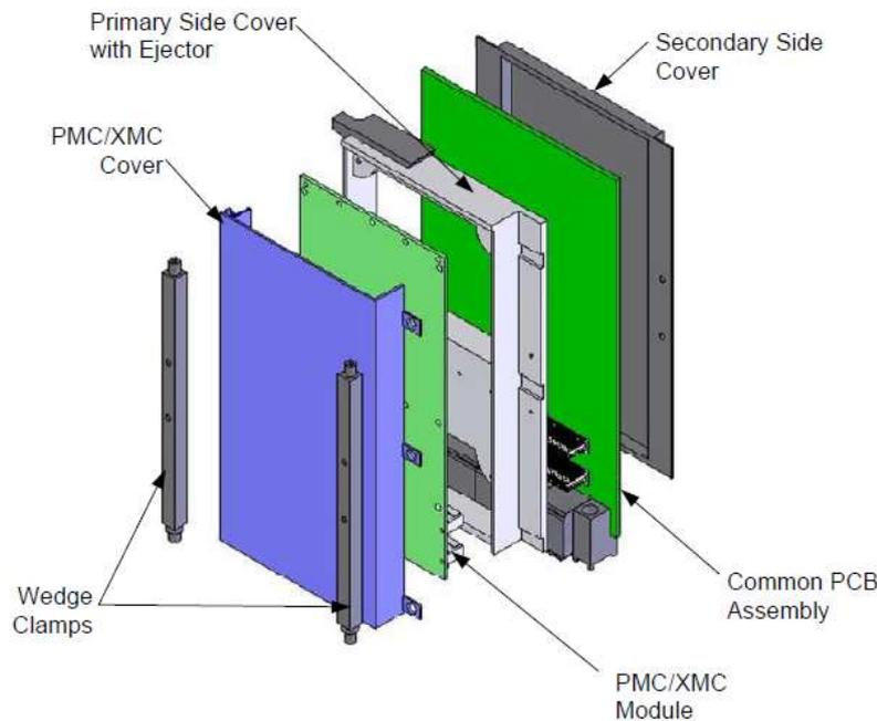
Figure 2: General configuration of 3U conduction-cooled plug-in units on 1.00 in centers [VITA Standards Organization, 2005]
