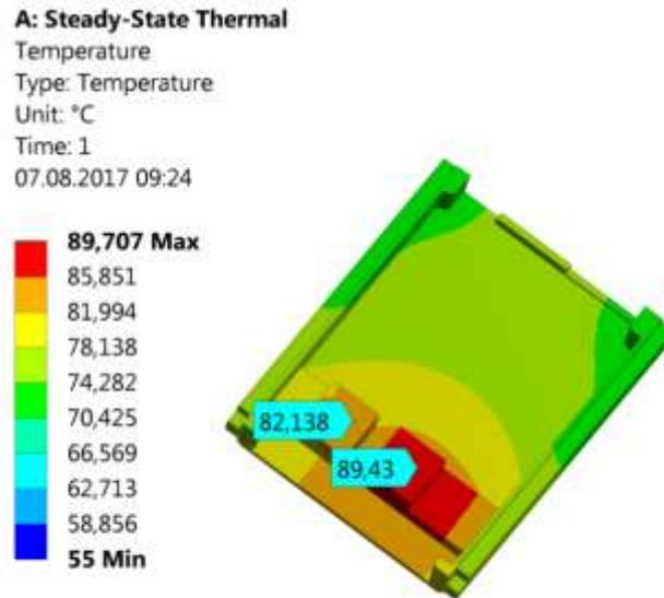
Figure 8: Temperature distribution in cpu cold plate
