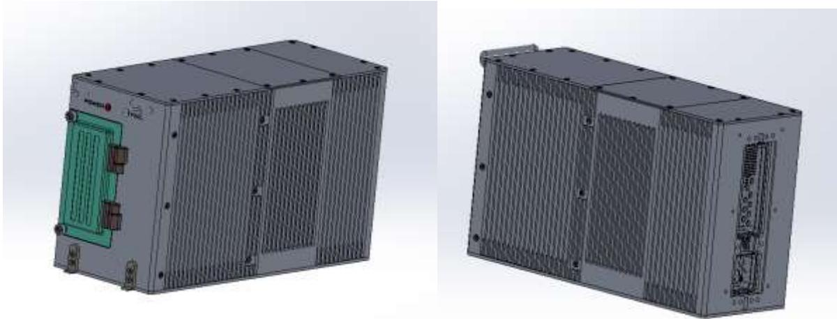
Figure 3: Draft design model of  $\frac{1}{2}$  atr chassis
