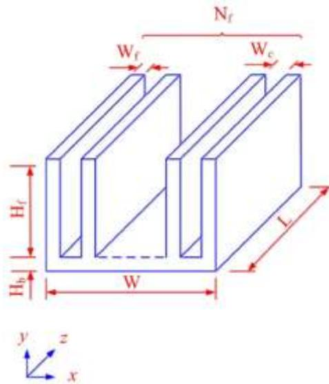
Figure 5: Geometric parameters of fin heat sink
