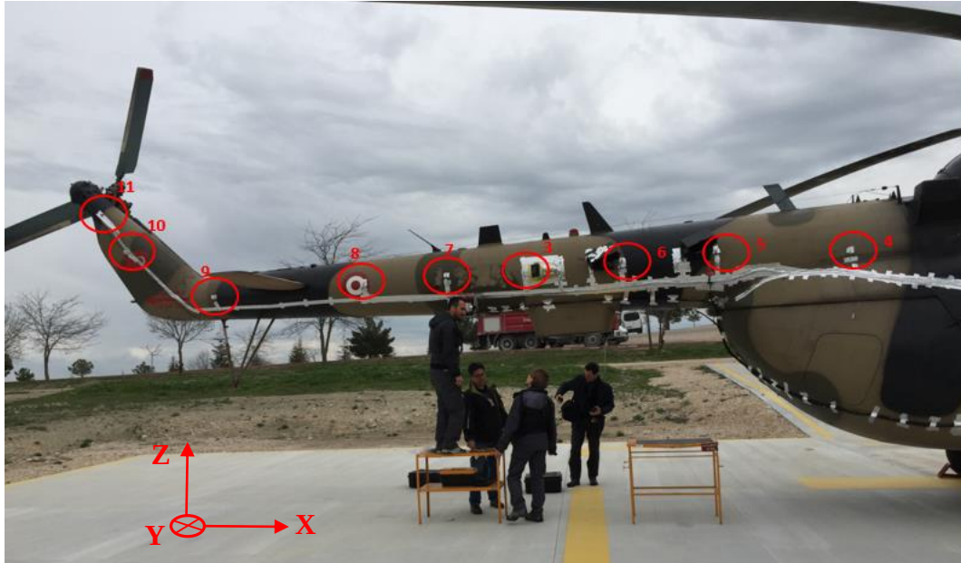
Figure 5: Operational Flight Tests Accelerometer Locations
