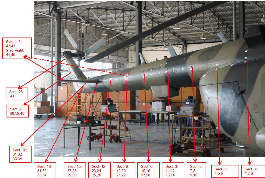
Figure 6: Ground Vibration Test Accelerometer and Shaker Locations
