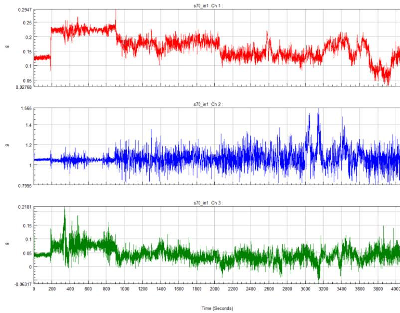
Figure 9: Time-dependent variation of maneuver (static) accelerations measured at the center of gravity of the helicopter at a normal flight (red: longitudinal / blue: vertical / green: sideways)
