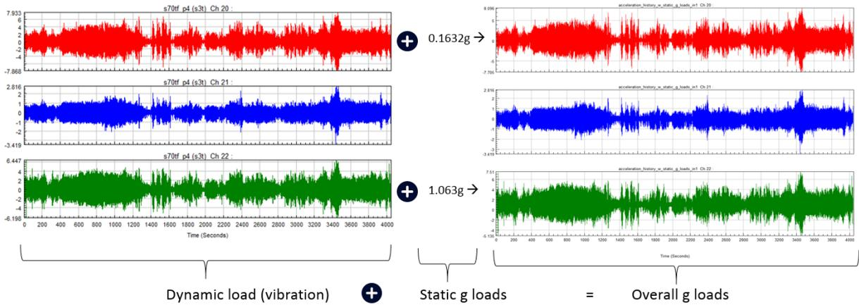
Figure 10: Total acceleration over a normal flight by gathering dynamic and static accelerations
