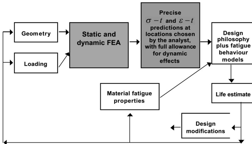
Figure 2: Finite Element Method Fatigue Analyzes [Bishop & Sherratt, 2000]
