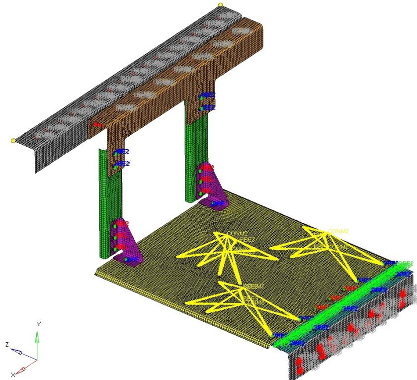
Figure 5: Finite element model of aluminum support carrying electronic equipment
