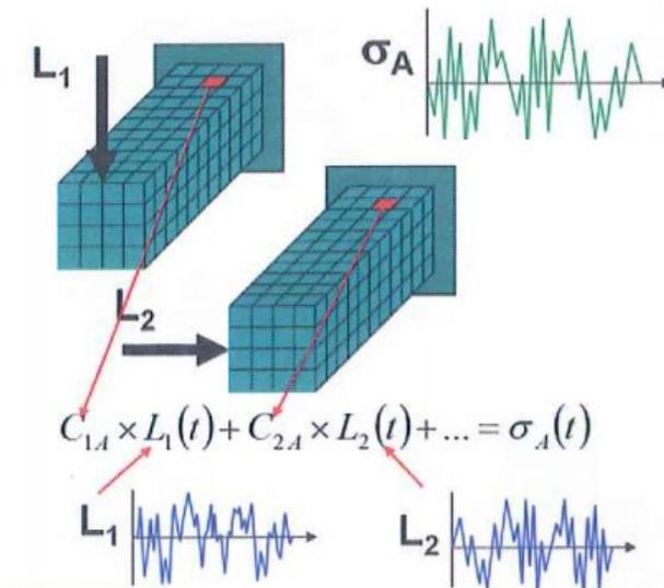
Figure 8: The accumulation of different loads in the time-domain fatigue method [ncode, 2010]
