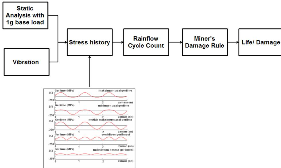
Figure 7: General flow of fatigue method in time domain
