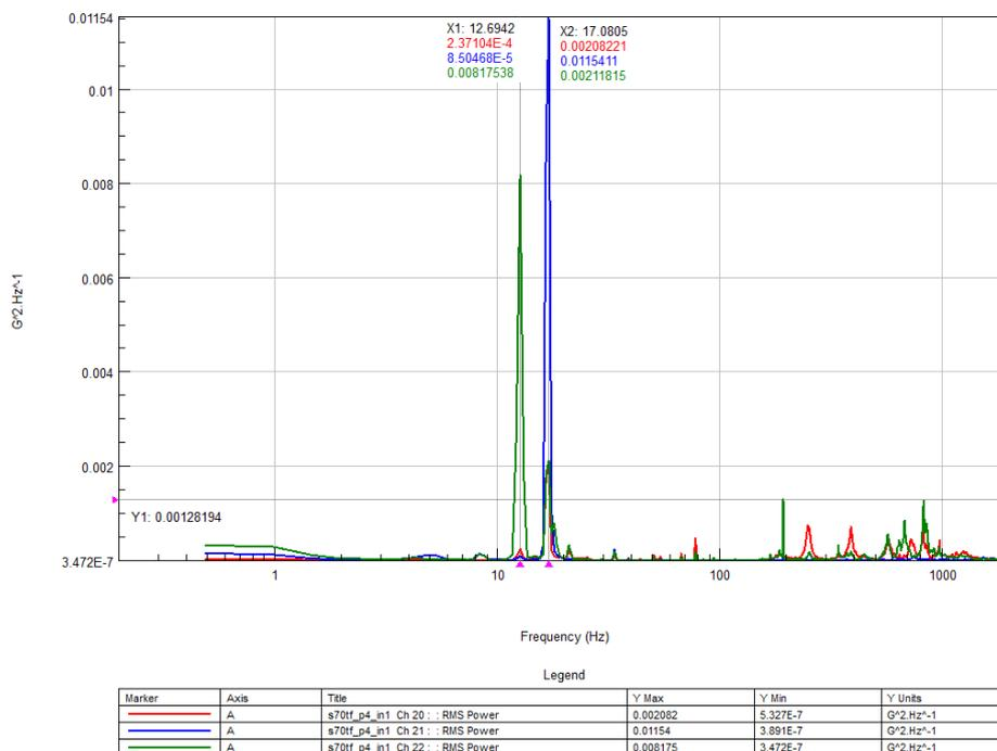
Figure 6: The power spectral density (PSD) of the vibration data measured
