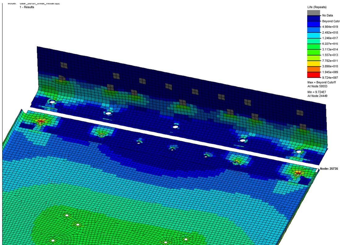
Figure 16: Fatigue analysis results of modal based transient dynamic analysis (time domain) method
