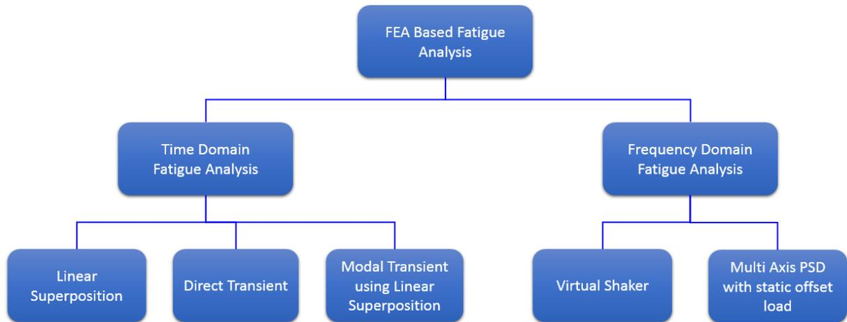
Figure 3: Different fatigue analysis types performed by means of finite element method in the frequency and time domain
