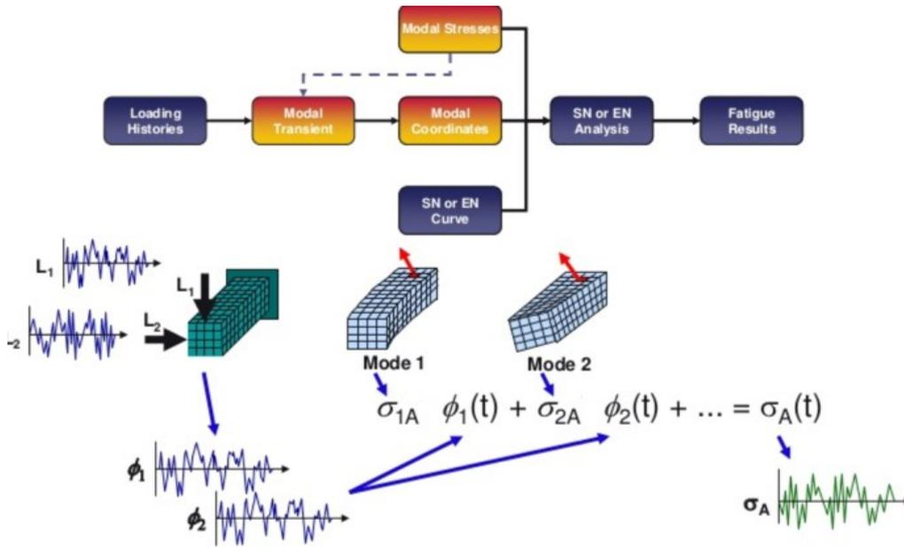
Figure 11: Fatigue Analyzes Using Modal Superposition Method [Vervoort, 2011]
