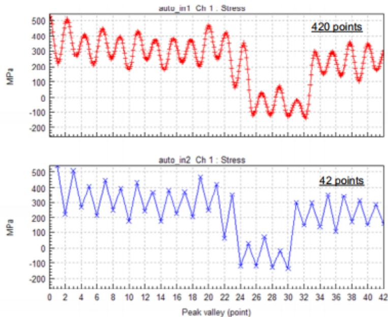
Figure 12: Simplification of load input in time-domain fatigue analysis with "Peak Valley" method [Halfpenny,2006]
