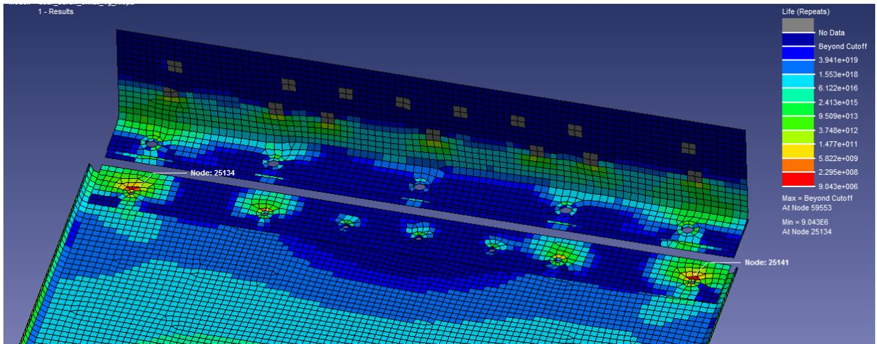
Figure 15: Fatigue Analysis Results of the linear superposition method (time domain)
