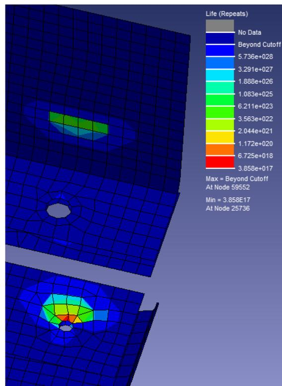
Figure 14: Fatigue analysis results of the multi-axis vibration (real conditions) (frequency domain)
