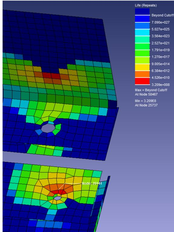
Figure 13: Fatigue analysis results representing the shaker test (frequency domain)
