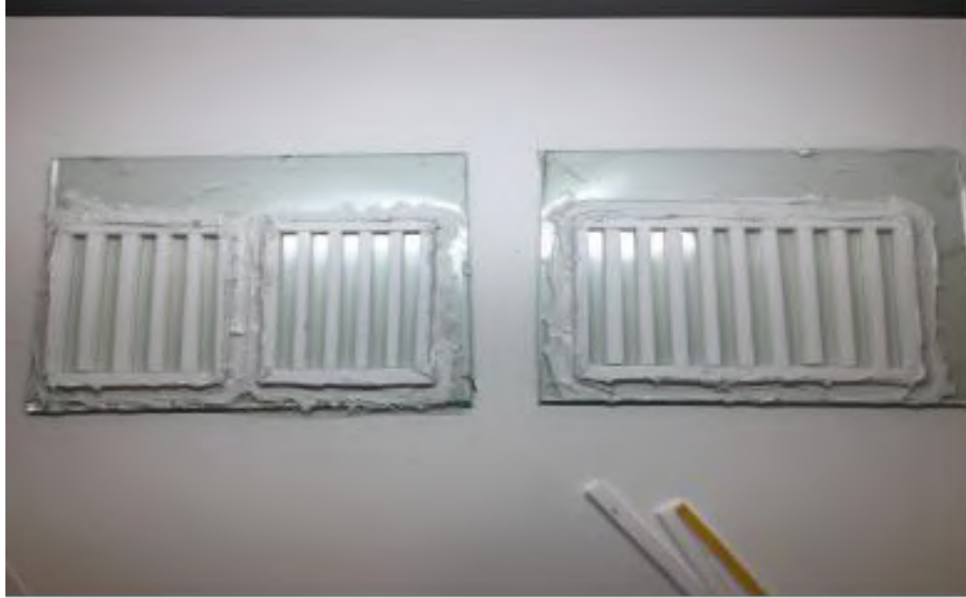
Figure 1: Teflon bars fixed on the Mylar® and surrounded with silicon
