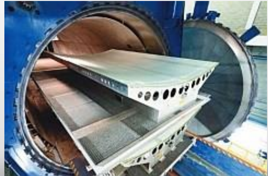
Fokker's traditional, non-automated production of GLARE fuselage panels
