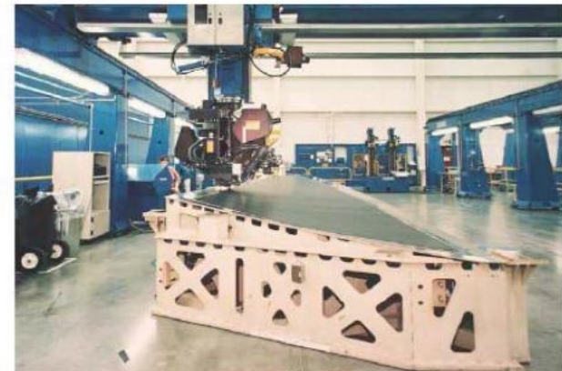
Boeing 777 Horizontal Stabilizer Skin Panel Lay up
