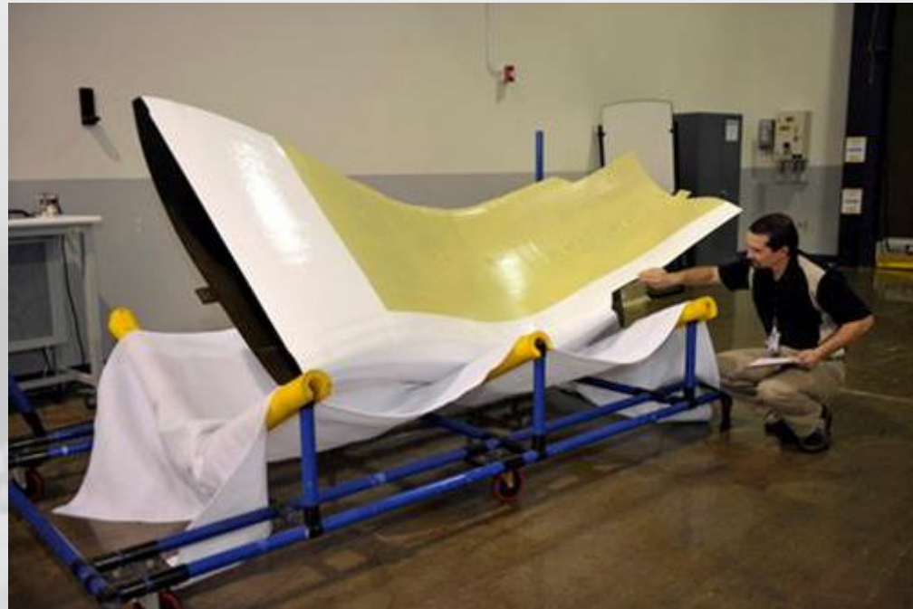
JSF Air-duct produced by AFP
