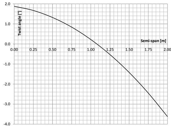
Figure 8: Twisted wing - Twist angle
