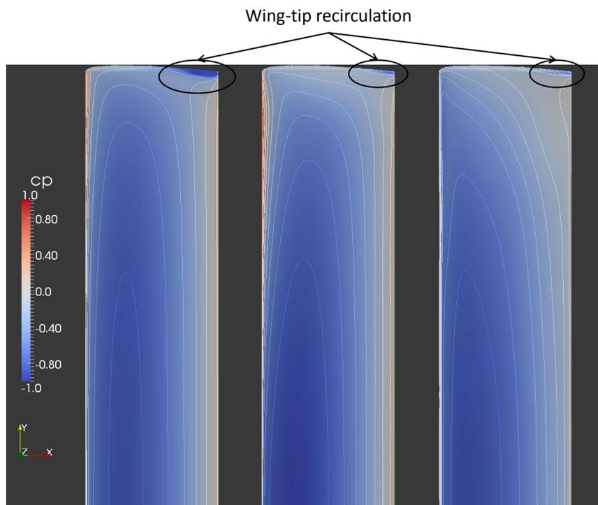
Figure 10: Pressure coefficient on the upper surface comparison
