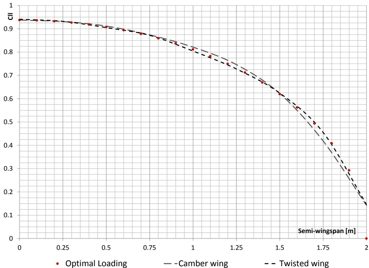
Figure 7: Spanwise optimal loading distribution
