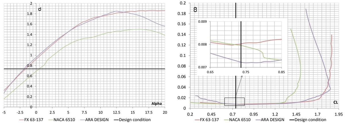
(a) Lift coefficient - alpha curve
