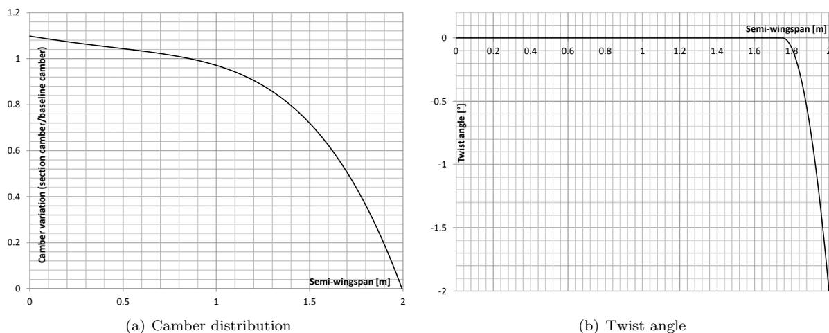
Figure 9: Cambered wing - Geometry
