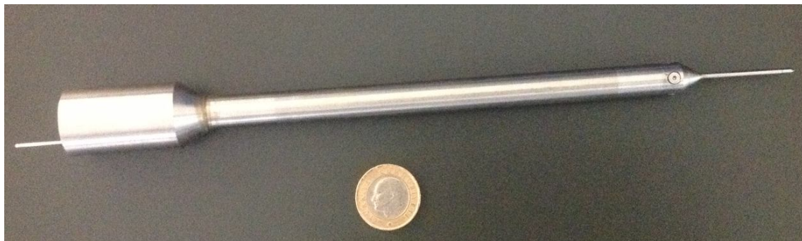
Figure 9 Fast response 5 hole probe manufactured by Aeroprobe Company
