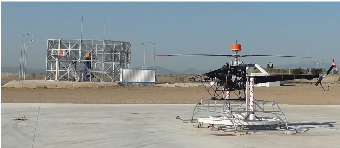
Figure 6 Designed rotor blade is installed on HC1 unmanned rotorcraft (400 kg MTOW)
