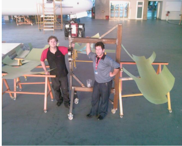
Figure 8: English Wheel Tool and Structural Maintenance Technicians
