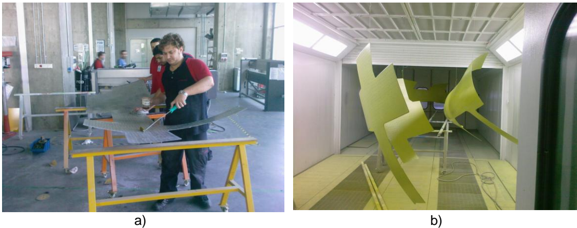
Figure 11: Preparation of Patches a) While Applying Protective Solution b) Patches in the Paint Drying Oven
