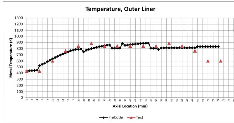
Figure 12: Comparison of PreCoDe and thermal paint test results
