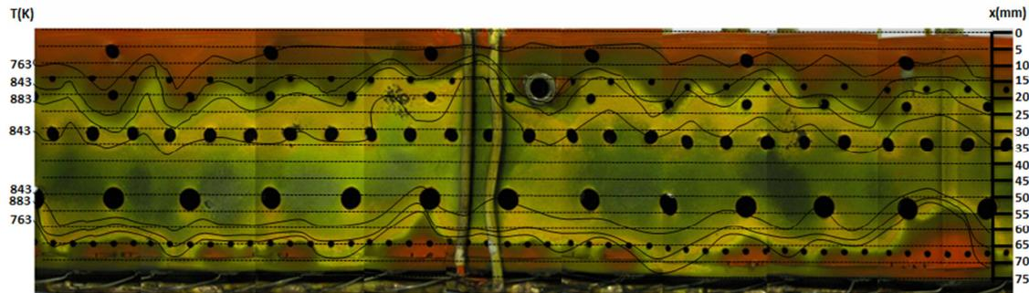
Figure 11. Thermal gradients of the combustor outer liner
