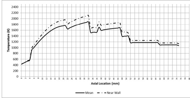
Figure 4: Mean and near wall gas temperature distribution along the axis of the combustor segment
