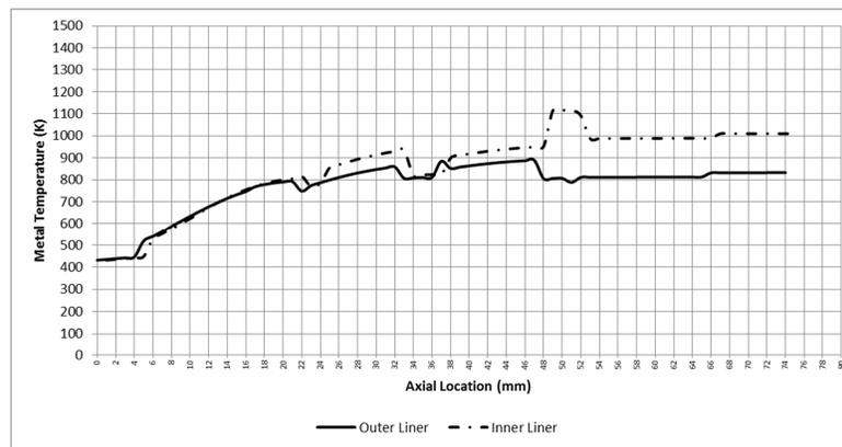
Figure 6: Wall temperatures for outer and inner liners
