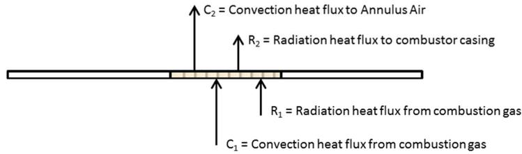
Figure 5: Basic heat transfer process in the combustor liner
