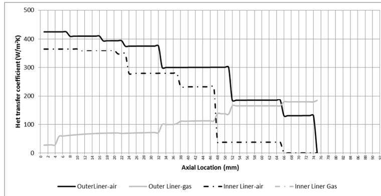
Figure 8: Heat transfer coefficients at the air and combustion gas side
