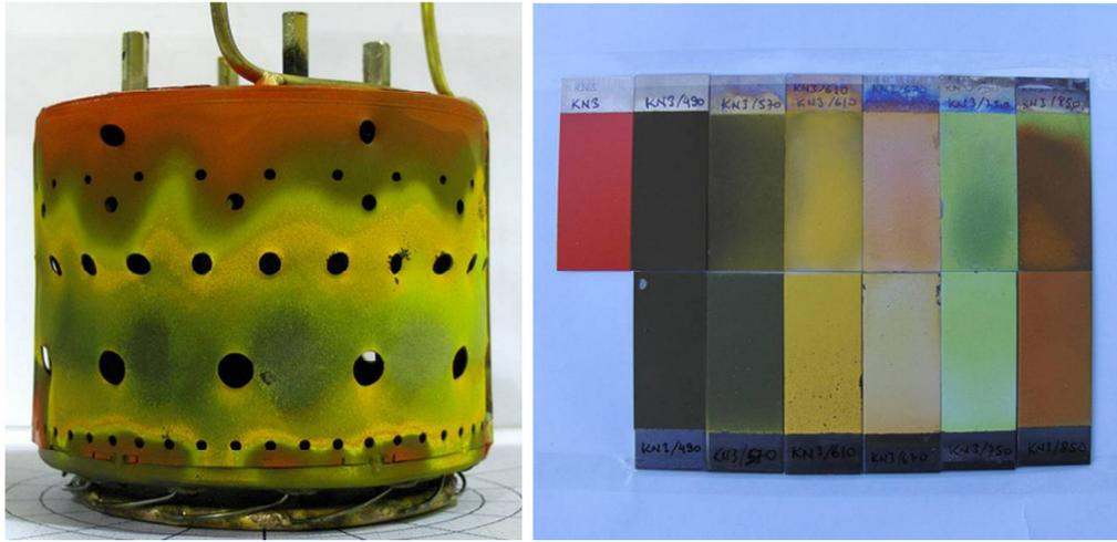
Figure 10: Thermal paint results of combustor and coupon scales
