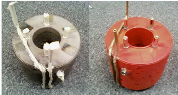
Figure 9: Thermal paint application on combustor
