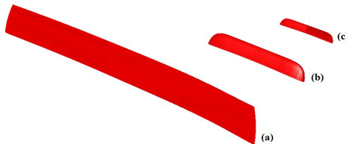
**Figure 10: (a) A finlet design sample; (b) 1<sup>st</sup> microvane design; (c) 2<sup>nd</sup> microvane design**
