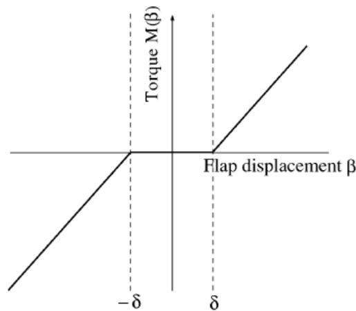
Figure 4: The Moment-Rotation Relation for a Free-play Nonlinearity Model [Liu, L and Dowell, E. H., 2005]
