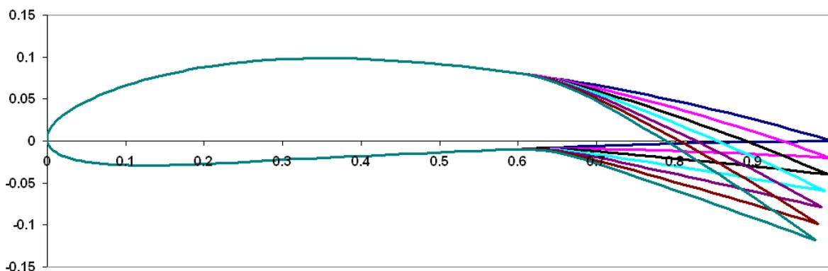
Figure 2: *Differential Shape Change of the Wing CS ( $\Delta f_k=0.0c$ ,  $\Delta f_k=-0.02c$ ,  $\Delta f_k=-0.04c$ ,  $\Delta f_k=-0.06c$ ,  $\Delta f_k=-0.08c$ ,  $\Delta f_k=-0.10c$ ,  $\Delta f_k=-0.12c$ )*[Yaman, Y., 2011]
