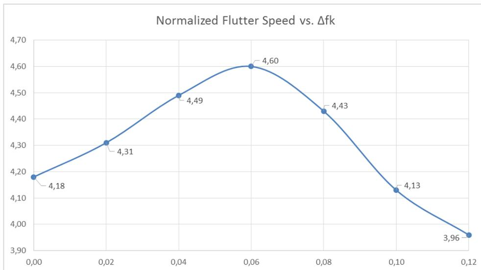
Figure 5: *The Effect of the Camber Change on the Nonlinear Flutter Speed*
