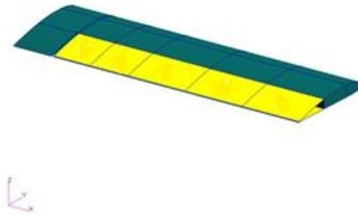
Figure 1: *Structural Model of the Wing*
