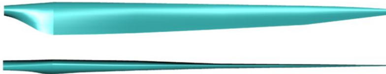
Figure 5 Blade Geometry of NordTank
