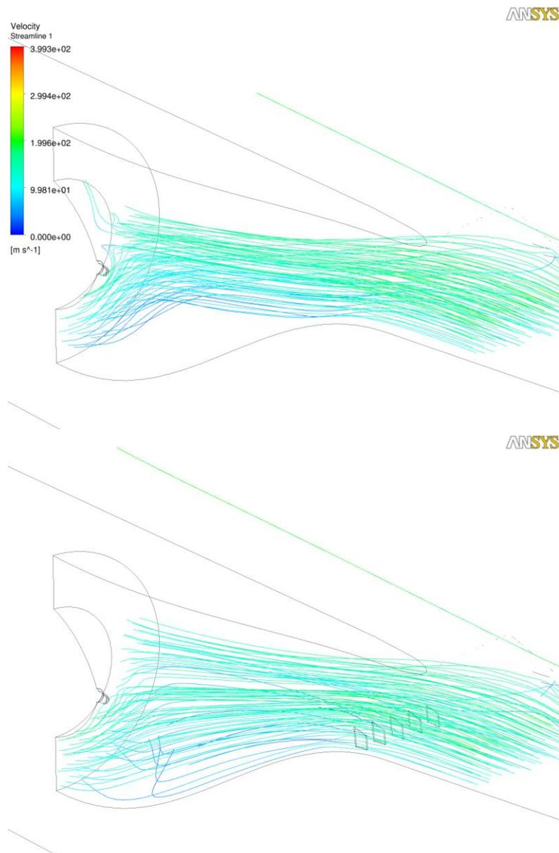
Figure 5: *Streamlines at engine duct. Top no vortex generators, bottom after application of vortex generators.*
