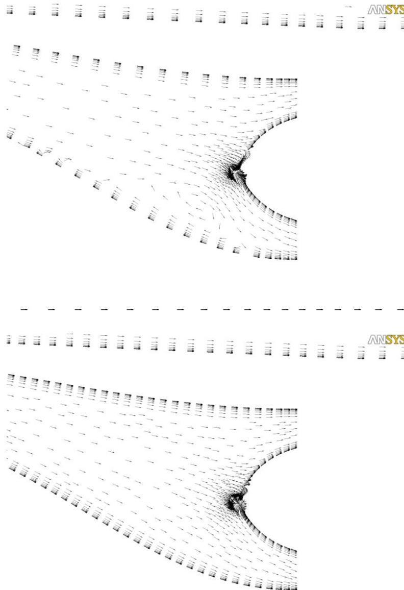
Figure 4: *Velocity vectors at engine duct symmetry plane. Top: no vortex generators, bottom: after application of vortex generators.*
