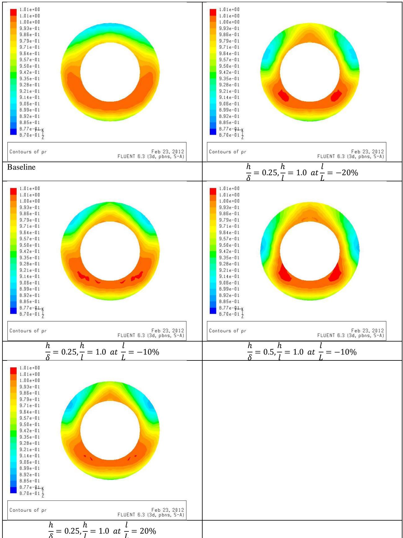
Figure 6: Total pressure distribution at engine inlet
