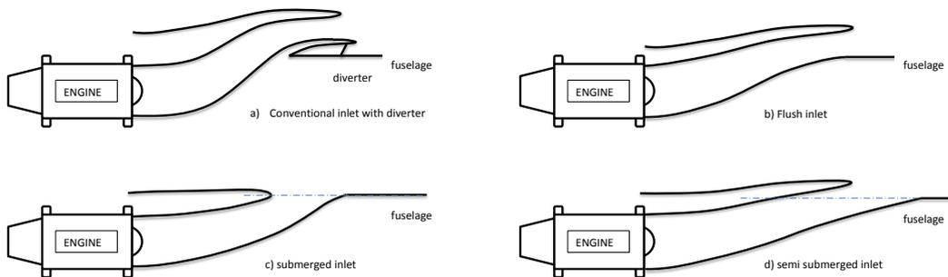
Figure 1: *Jet Engine Inlet Types by installation method used in Cruise Missiles*
