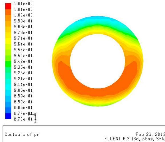
Figure 2: Typical total pressure distribution for diverterless inlets with no flow control.
